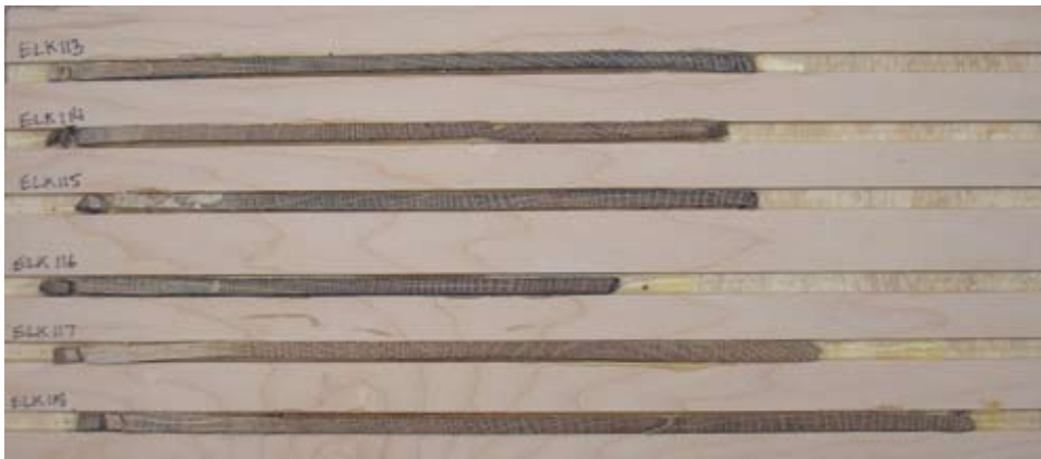
Figure 3.14 Tree ring cores can be used to assess disturbance and changed conditions at a site over the life of the tree. Cores can be taken with an increment borer, mounted, sanded, and viewed with a microscope. Software that measures each annual tree ring is useful for accurately recording small variations in growth and creating site chronologies. Photo: Shyanne Smith
