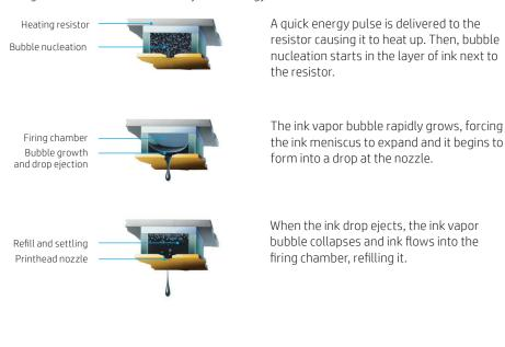
Firing a nozzle with HP Thermal Inkjet technology
