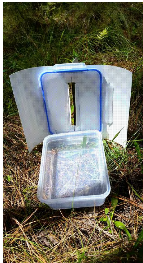
Figure 3. Opened burrow facade trap showing slits that specimens fall through and container beneath
