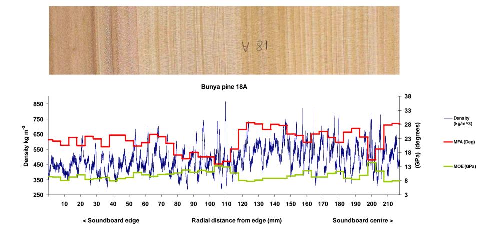
**Appendix 5** Silviscan-derived wood properties and corresponding strip from soundboard half
