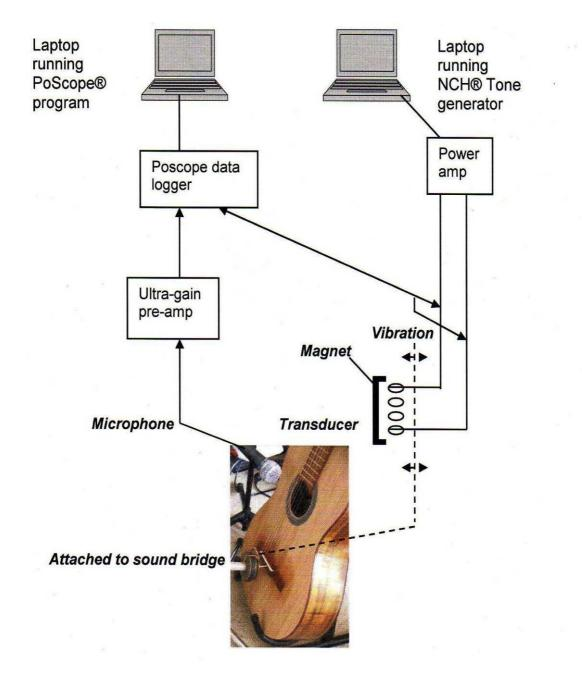
Figure 43. Schematic diagram of spectral analysis used in the objective evaluation of instruments (Equipment and methodology provided by Mr David Chin)
