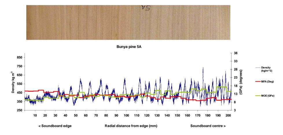
Appendix 6 Silviscan-derived wood properties and corresponding strip from soundboard half
