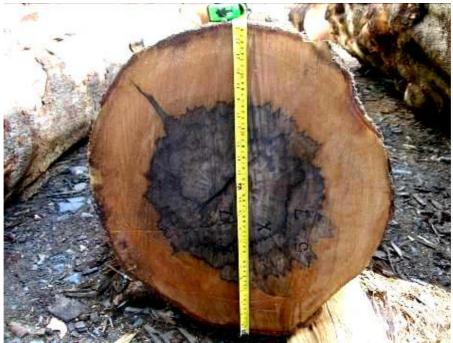
Figure 17. Blackheart sassafras log – 60cm large end diameter
