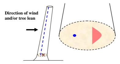
Figure 25.Compression wood zone indicated in red. The off-centre pith (blue line) can be indicative of a compression wood zone within the large radius.
