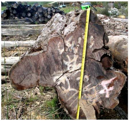
Figure 24. Older buttressed blackwood logs are more likely to produce fiddleback material in the lower butt. (Corinna Sawmill, Burnie Tasmania 2007.)
