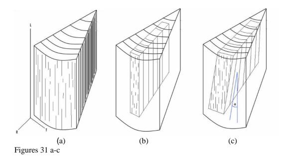
Ideally grain in longitudinal plane (L) provides the reference for all subsequent breakdown cuts. As previously mentioned it is also desirable to have growth rings as close to perpendicular to the wide face of the board as possible (i.e. fully quartersawn).
