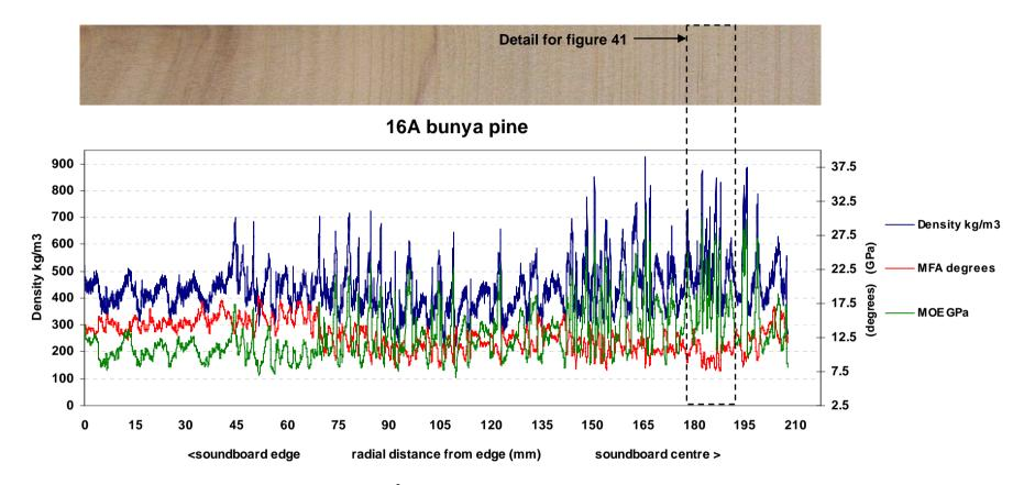
Figure 38 Plate 16 (guitar four) Mean: density 440 kg/m<sup>3</sup> - MOE 12.7 GPa - MFA 13° - along grain sound veloc ity 5674 m/sec.
