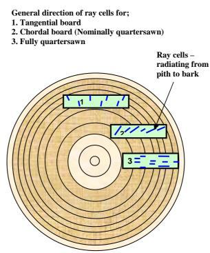
Figure 29. Ray cell direction in 1. backsawn, 2. nominally quartersawn and 3.fully quartersawn boards
