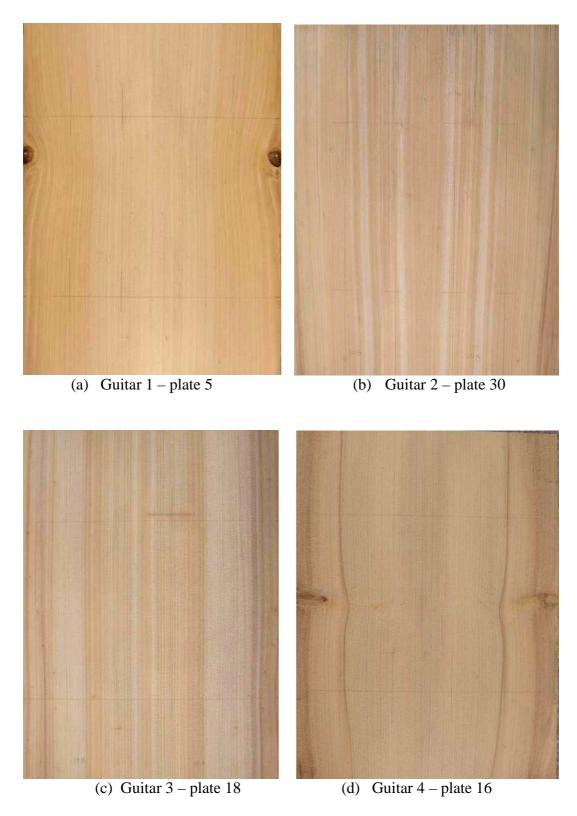
Figures 37 a-d The four bunya pine soundboard plates used in the evaluation.
