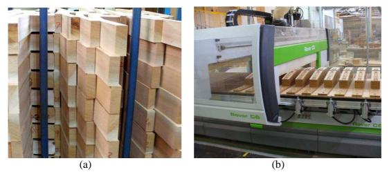
Figures 7 a-b. Queensland maple acoustic guitar neck blanks and one of two new CNC routers (Maton Guitars 2008)
