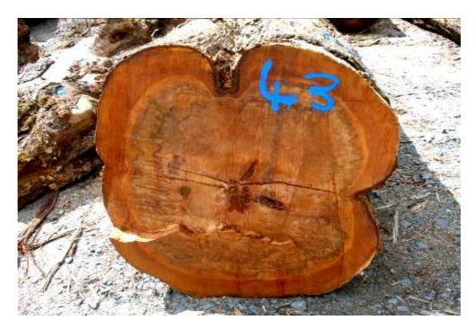
Figure 20. Myrtle log (without tiger colouration) 1.1m diameter large end Part of log tender at Forestry Tasmania's Island Specialty Timbers in Geeveston.
