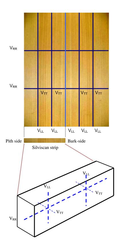
Figure 36 Measurement points on soundboard plates and Silviscan strips.
