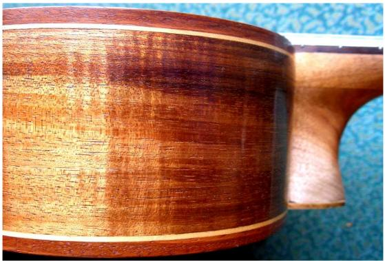
Figure 8. Blackwood guitar side with jarrah and huon pine bindings
