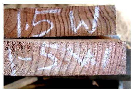
Figure 14. Silver wattle (*Acacia dealbata*) 150mm wide boards with around 24 years of growth within the board width (Phillips Sawmill, Geeveston 2007)
