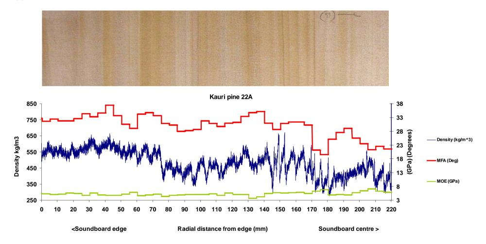
**Appendix 8** Silviscan-derived wood properties and corresponding strip from soundboard half
