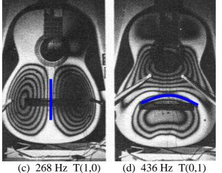
Figures 44 a-d Hologram interferometery (Images from Richardson 1994). Blue lines showing nodal (non-moving) region.
