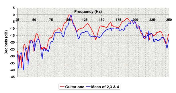
Comparison of Sound pressure level (dB) -Guitar one vs. mean of guitars two, three and four
