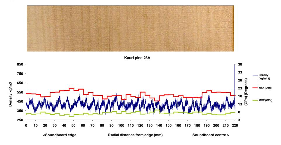
Appendix 7 Silviscan-derived wood properties and corresponding strip from soundboard half
