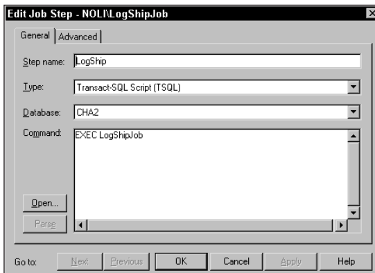
Figure 29-4: A SQL Server Agent job executes the LogShipJob stored procedure every five minutes.
