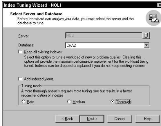
Figure 28-8: The Index Tuning Wizard can keep existing indexes and offers three levels of analysis.
