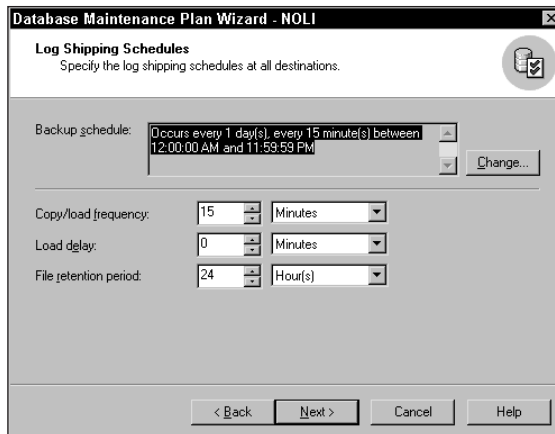
Figure 29-2: The log-shipping backup and handling schedule is created in the Log Shipping Wizard.
