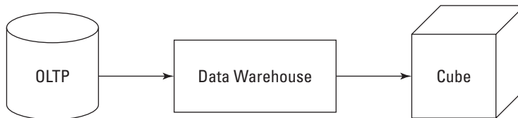
Figure 31-1: The process the data will travel before finally being stored in a cube.
