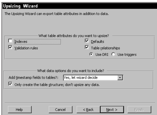
Figure 3-4: The Access Upsizing Wizard can move the schema and data to a SQL Server database.
