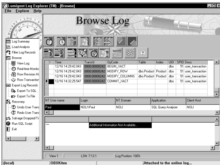
Figure 11-8: The commit entry is written to the transaction log, just as the data modifications were.
