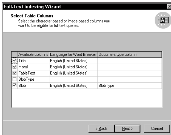
Figure 8-2: Any valid columns are listed by the Full-Text Indexing Wizard and may be selected for indexing.
