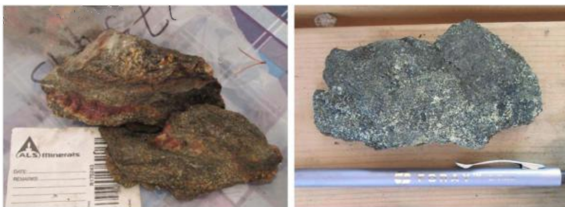
Figure 19 - Left : Sample 175243 returned 1.6% Cu, 21.2 g/t Ag and 2.9 g/t Au in a paragneiss. Right Chalcopyrite heavy disseminations in an amphibolite (Sample 175300, 4.77% Cu, 1.49 g/t Au).
