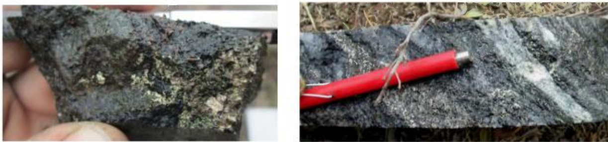
Figure 18 - Details of sample 175110 Ni-Cu mineralisation returning 0.306 % Cu, 0.466 % Ni and 0.23 g/t Pd
