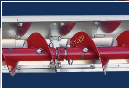
New splice plate for added strength
