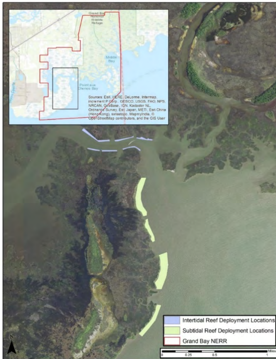
Figure 22. Priority areas selected for construction of sub- and intertidal reefs within the GNDNERR. The polygons show the areas being permitted for reef construction, which are larger than the final project area.
