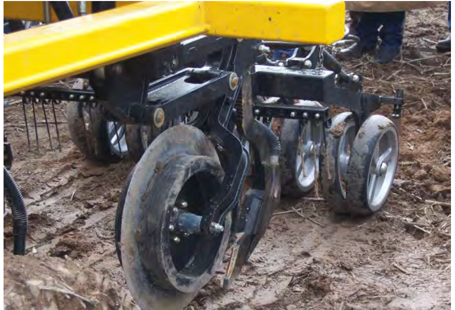
Photo 9: A Bio Blade or Cross slot™ disc opener with opening disc and seeding tyne, followed by paired press-wheels. Note that the seed and fertiliser tube has sharp bends and may not be wide enough to avoid blockages when larger-seeded pulses like faba or broad bean are being sown.
