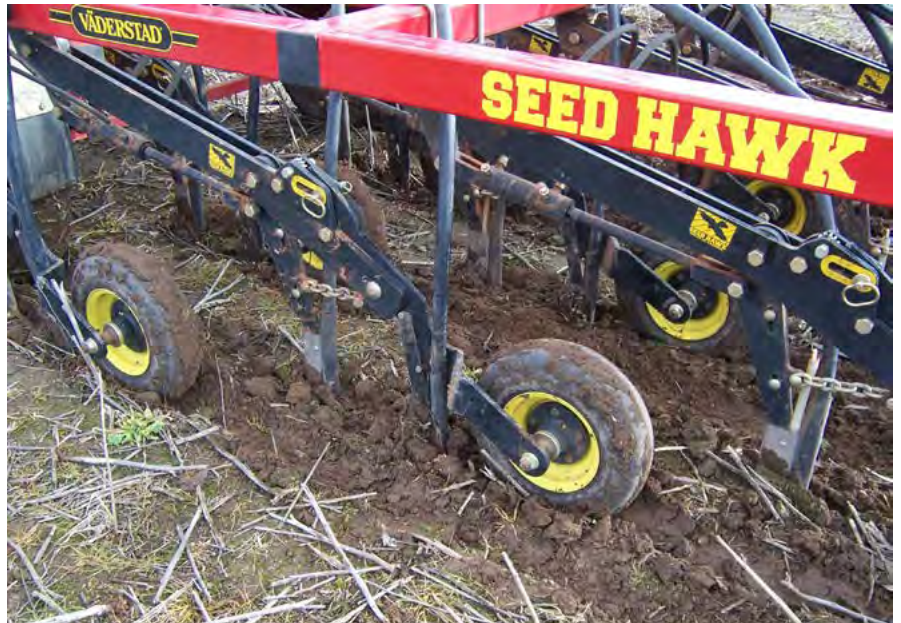
Photo 8: One of several seeding mechanisms for uniform sowing depth using the press-wheel for depth control.
