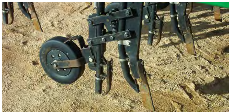
Photo 6: The DBS system parallelogram for uniform seeding depth and deep placement of seed or fertiliser.
