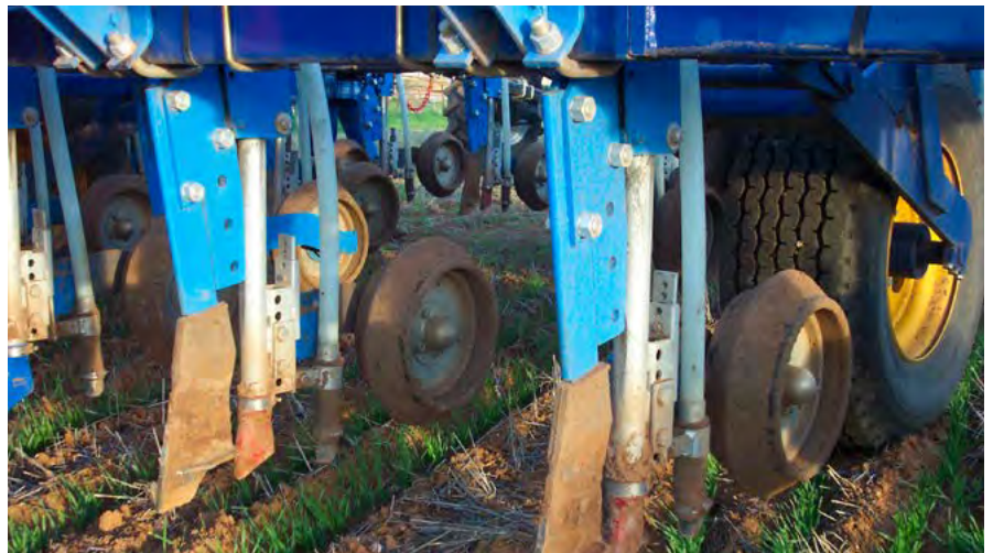
Photo 5: A Primary Precision Seeder fitted with hydraulic breakout for consistent penetration. It is also fitted with narrow points that form an 'inverted T' slot. It is capable of deep or side placement of fertiliser.
