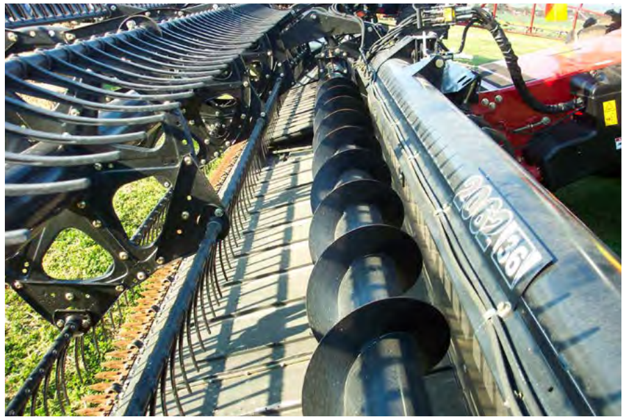
Photo 7: Belt front fitted with cross auger.
