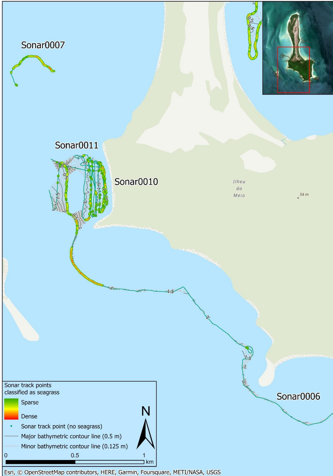
Figure 67 : Bathymetric contours and seagrass presence derived from sonar data gathered in Meio's coastline (Sonar0006, Sonar0007, Sonar0010 and Sonar0011 transects). Seagrass presence colour ramp represent the relative density of points classified as seagrass (i.e. the relative density is based on point count).
