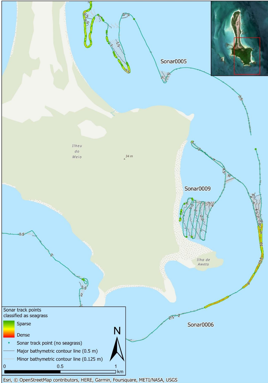
Figure 66 : Bathymetric contours and seagrass presence derived from sonar data gathered in Meio's coastline (onar0005, Sonar0006 and Sonar0009 transects). Seagrass presence colour ramp represent the relative density of points classified as seagrass (i.e. the relative density is based on point count).
