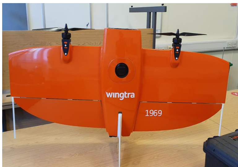
Figure 5 : Wingtra VTOL fixed-wing drone. Nose cone is not included in this image.
