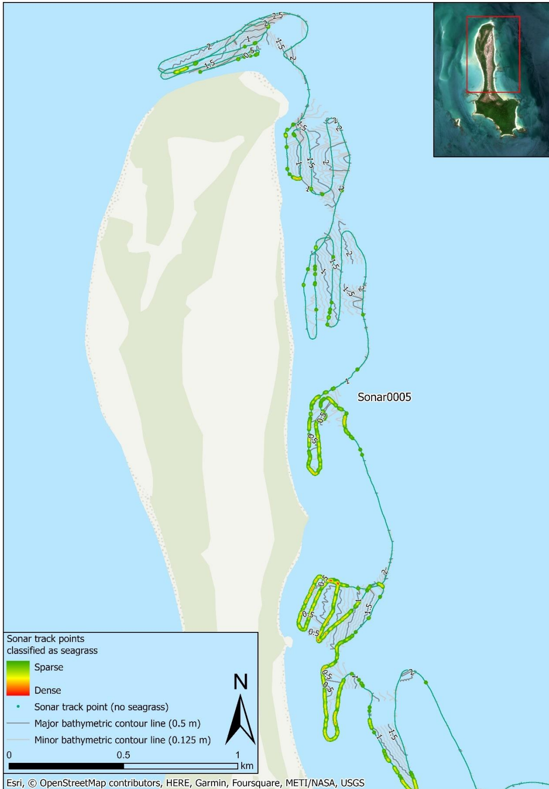
Figure 65 : Bathymetric contours and seagrass presence derived from sonar data gathered in Meio's coastline (Sonar0005 transect). Seagrass presence colour ramp represent the relative density of points classified as seagrass (i.e. the relative density is based on point count).
