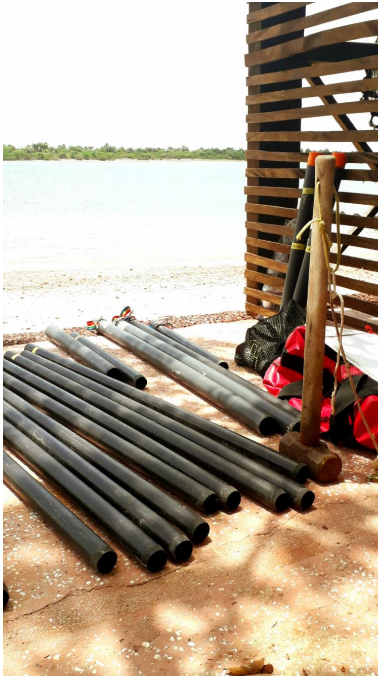
Figure 38 : PVC pipes used to collect the sediments in Unhocomozinho, Guinea-Bissau, August 2022. Photo: G. Touron-Gardic
