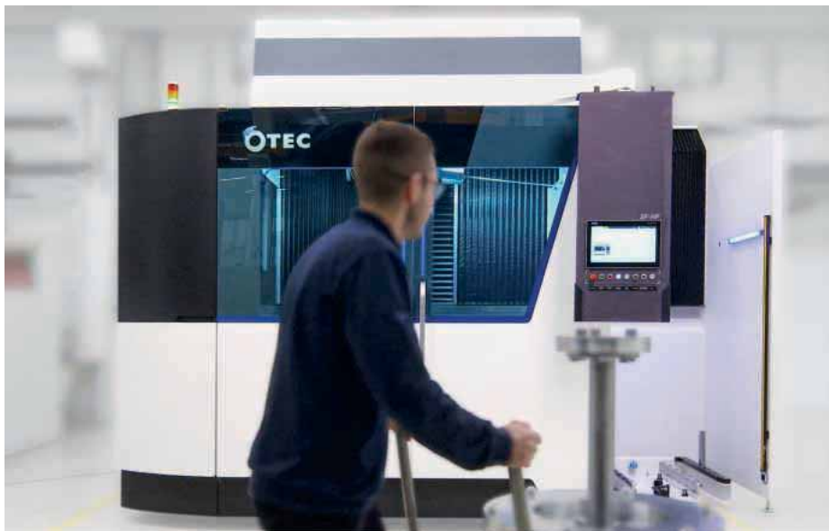
Loading an OTEC SF-HP, bringing the company's stream finishing technology to larger aerospace parts and more
