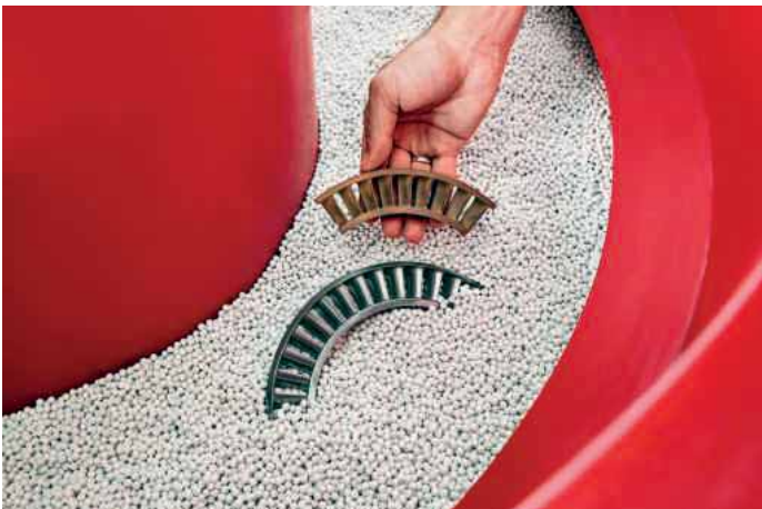
A 3D printed blisk segment (top) and after the "Trowalizing" process
