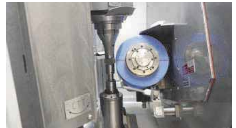
Kapp Niles - generating grinding process
