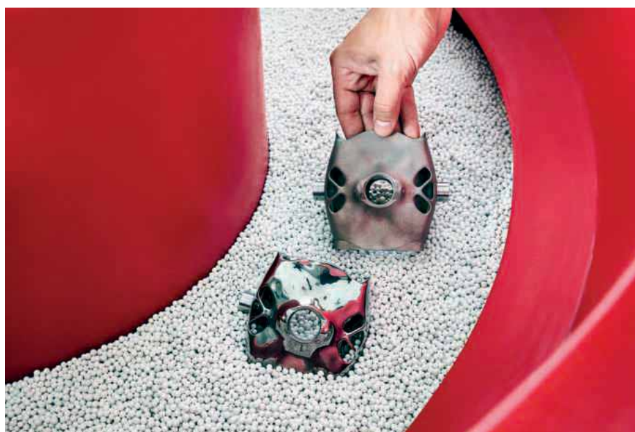
A 3D printed gimbal frame before (top) and after the "Trowalizing" process
