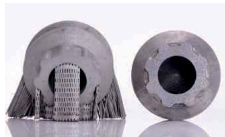
An additive part with support structures, before and after Hirtisation
