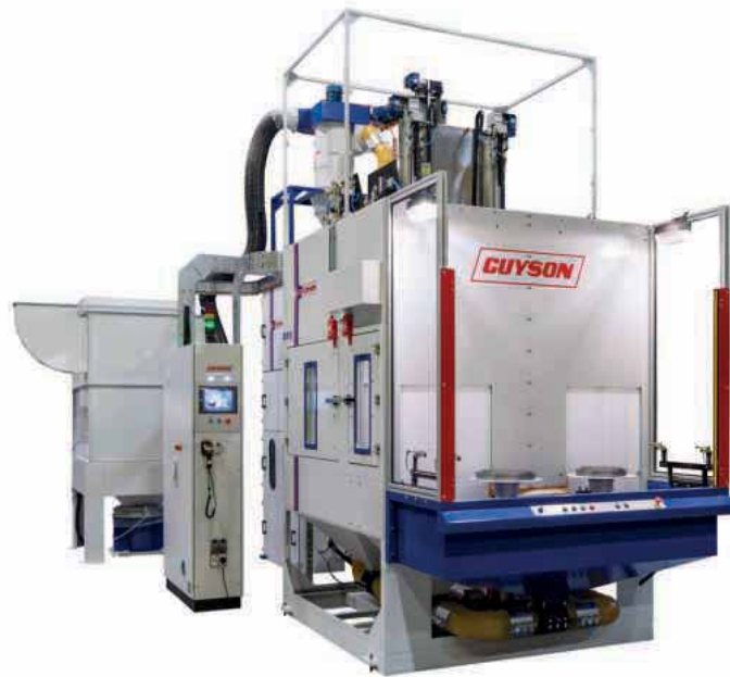
Guyson Multiblast RXS1400 automated blast cabinet with cyclone and dust collector
