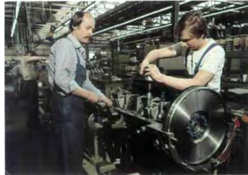
Assembly of heavy commercial vehicle engines at our Berlin-Marienfelde plant: Here the crankshaft is being fitted.
