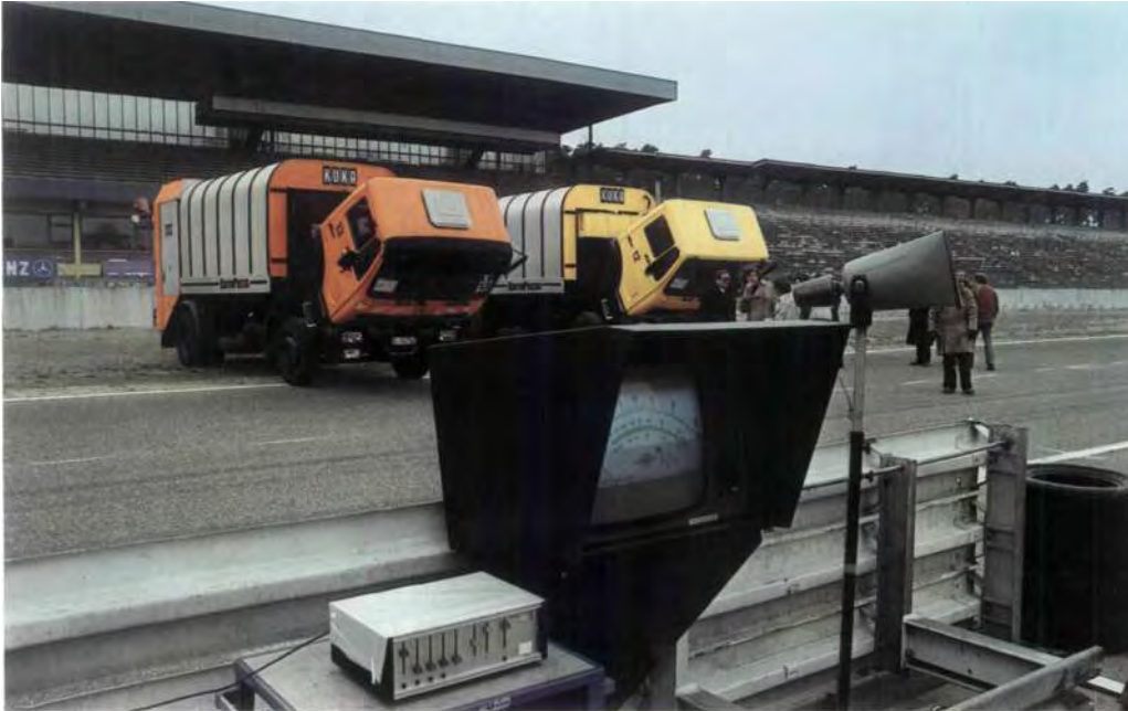
Quiet commercial vehicles with encapsulated power plants - demonstration of the results achieved to date of a research project at the Hockenheim Motodrome in November, 1981.
