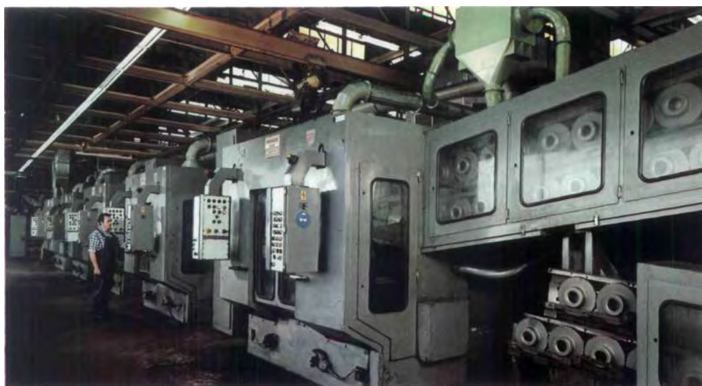
The only manual operation is loading: fully automatic interconnected lathe transfer system for machining of front wheel brake discs at the Mettingen plant.
