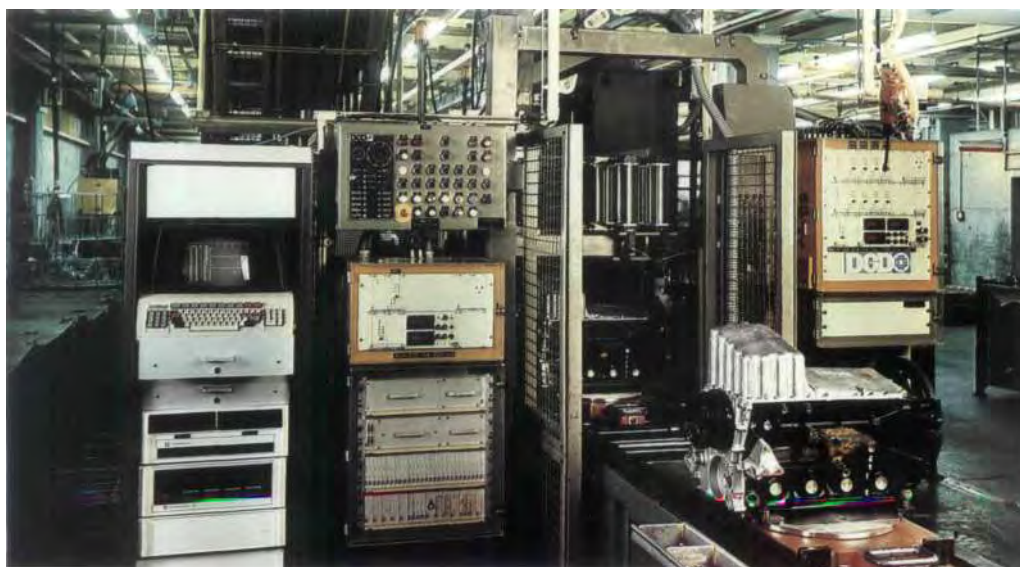
Electronically controlled automatic bolting station in car engine assembly at the Untertuerkheim plant.
