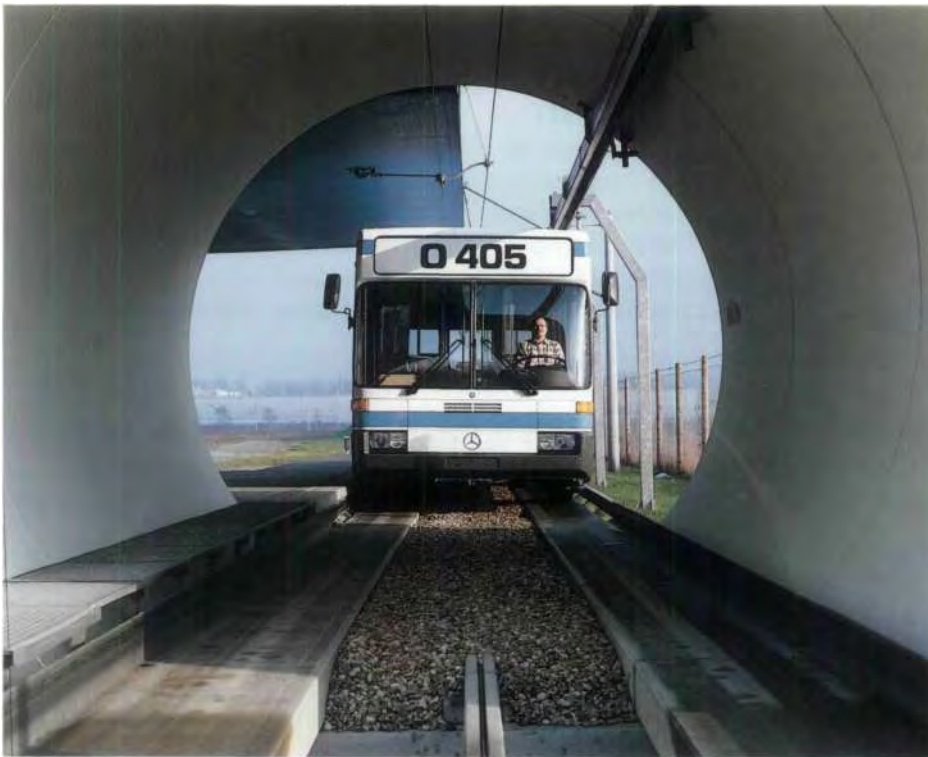
The new track-guided standard city bus O 405 on the company's test track in
