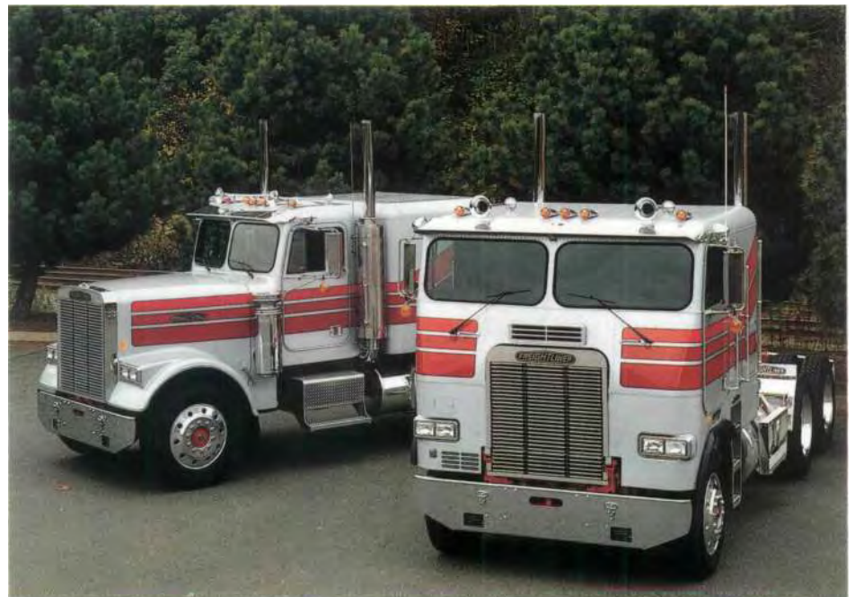
The heavy-duty conventional and the heavy-duty COE tractor are the two basic models of
