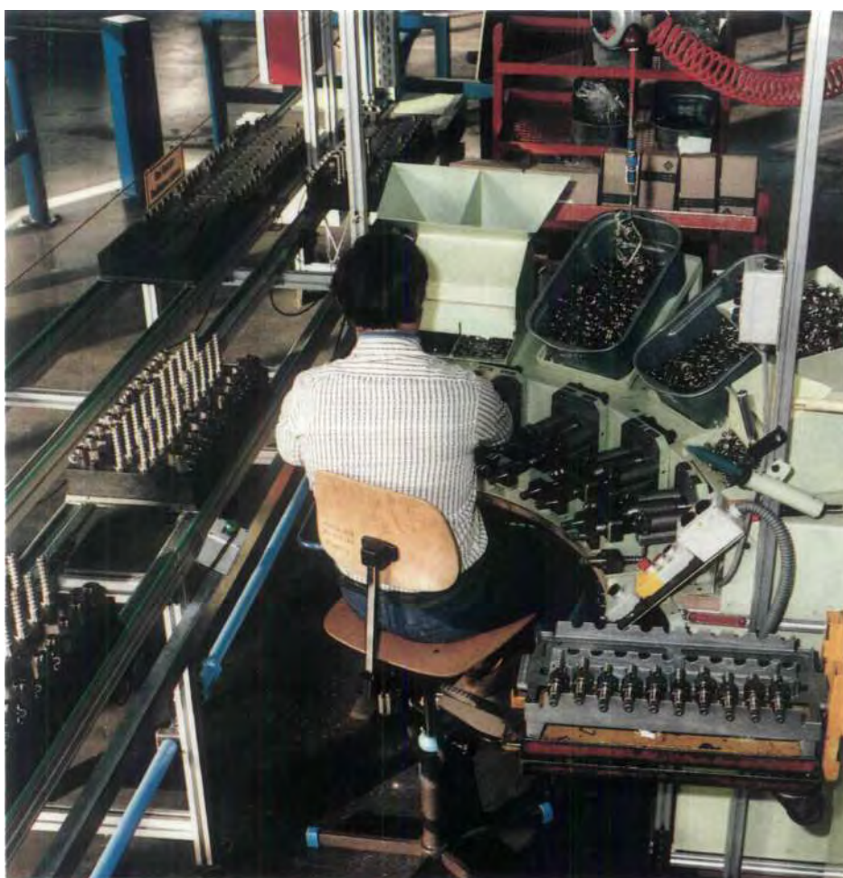
At the Duesseldorf factory: An economically optimized assembly station in steering unit assembly. The semicircular arrangement
