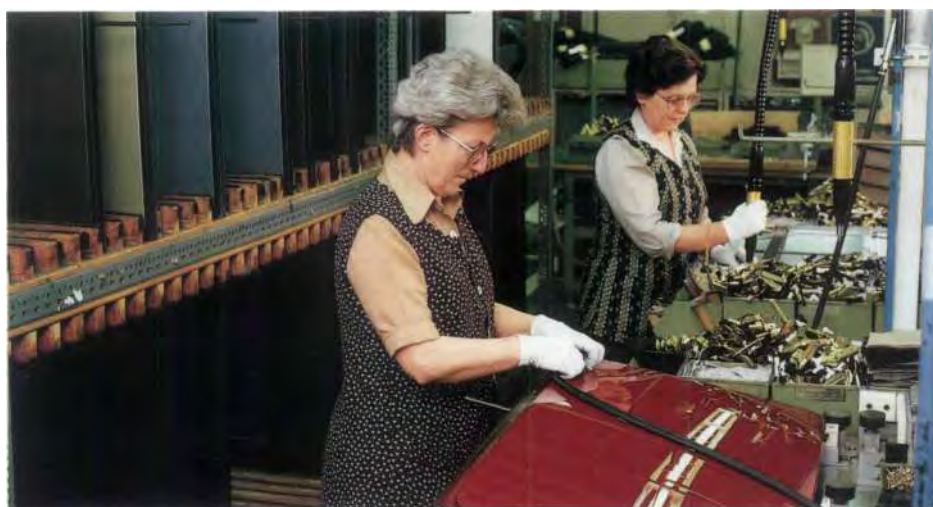
Modern work methods help reduce strain. Example: individual workstations in sunroof preassembly are independent of line speed.
