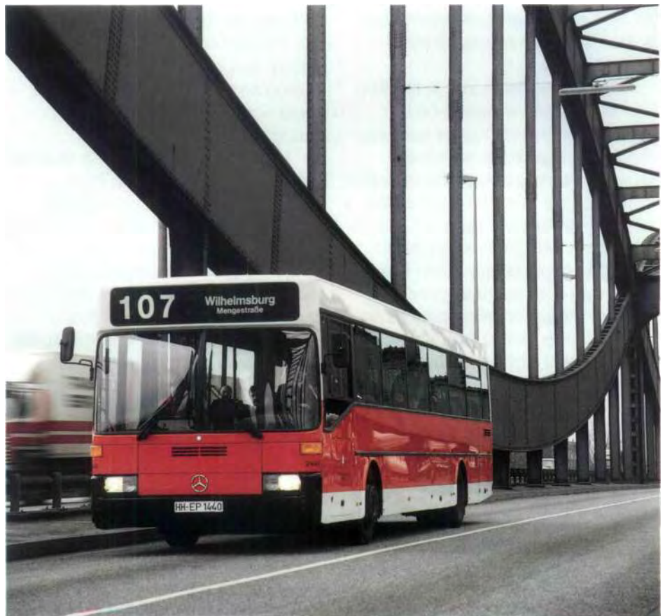
The new standard city bus O 405 for intra-city transportation. It can carry 100 passengers. The new series also
