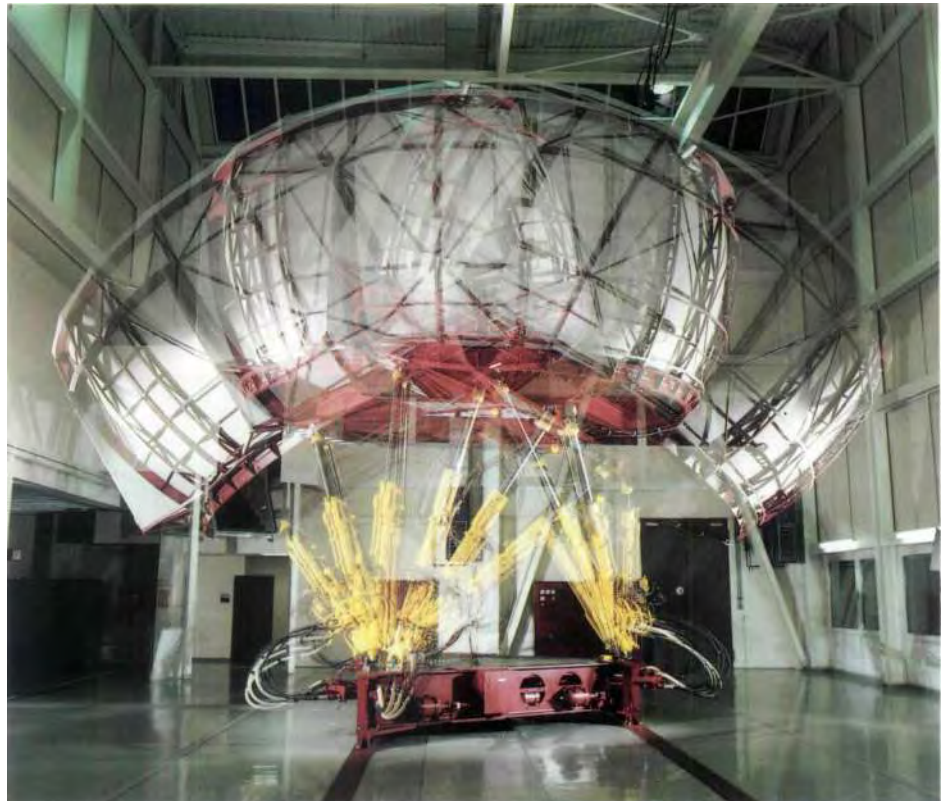
The new driving simulator at the Berlin-Marienfelde factory. Aided by a mathematical model of a vehicle, a computer controls all the movements of the cabin in such a way that the driver gets the im-
