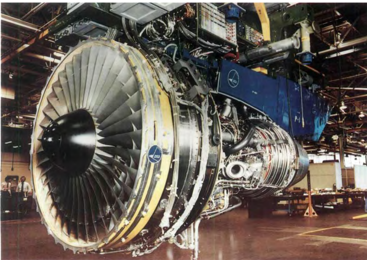
The turbo fan power plant PW 2037 brought to fruition by MTU in cooperation with Pratt & Whitney resulted in the assumption of responsibility by MTU for the development and manufacture of a complete module, the low pressure turbine.
