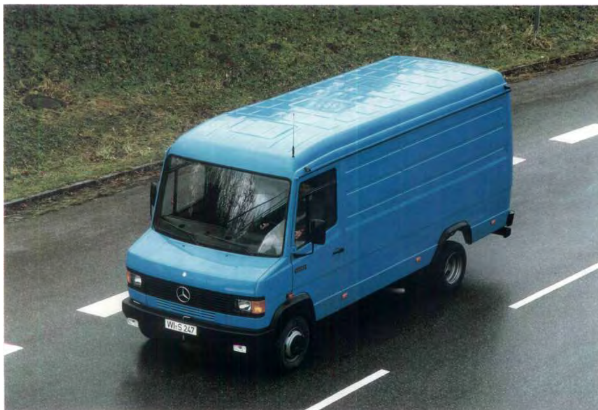
The new series T 2 delivery van is based on the engineering concept of light-weight trucks from Woerth; the model range extends from 4.6 tons to 7.5 tons of permissible gross vehicle weight and also comprises variations allowing lesser loads.
