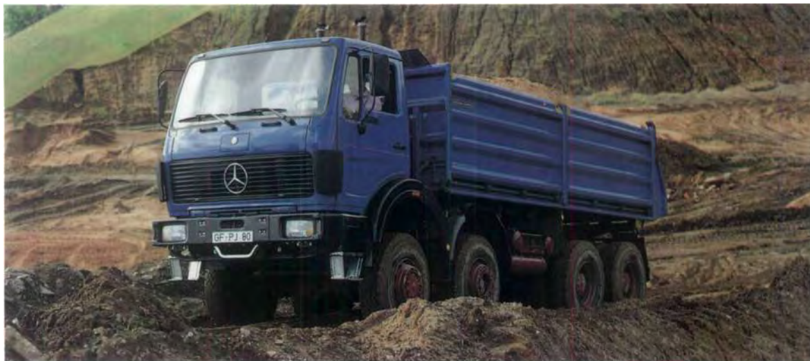
Mercedes-Benz heavy-duty truck of our Swiss partner NAW. The particularly robust components, such as large-volume suction engines and planetary hub reduction axles, withstand the test in off-the-road operation.
