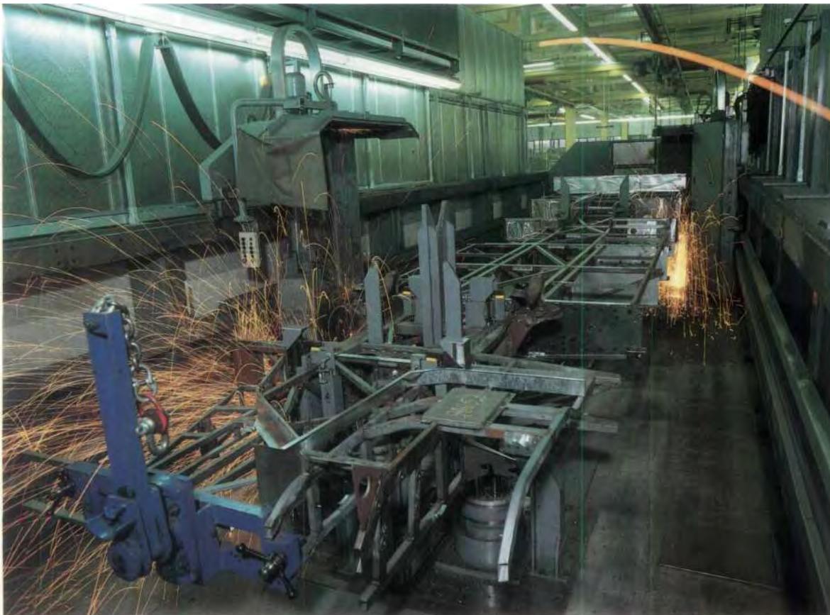
Accurate measurements are a sign of quality in the manufacture of Mercedes-Benz buses. The picture: a trim station for bus undercarriages at the Mannheim plant.
