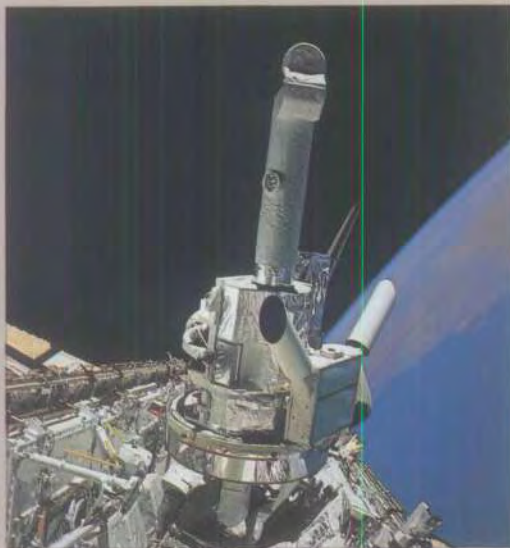
The "Instrument Pointing System" (IPS) is a precise alignment system, used in the Space Shuttle Program. It was designed and produced by Dornier by order of the European Space Agency (ESA).
