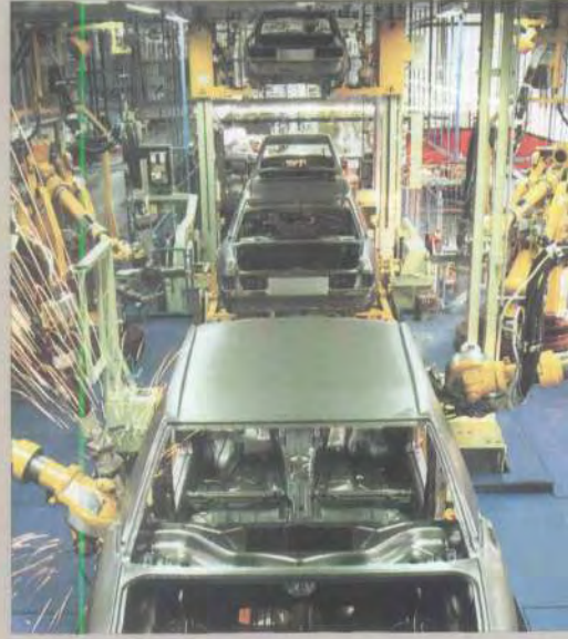
Industrial robots assure consistently high precision standards in body shell construction and free man from heavy manual labor.
