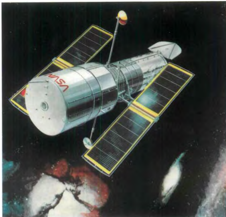
Space telescope of NASA with roll-out solar generator which has a power rating of 4 kW.
