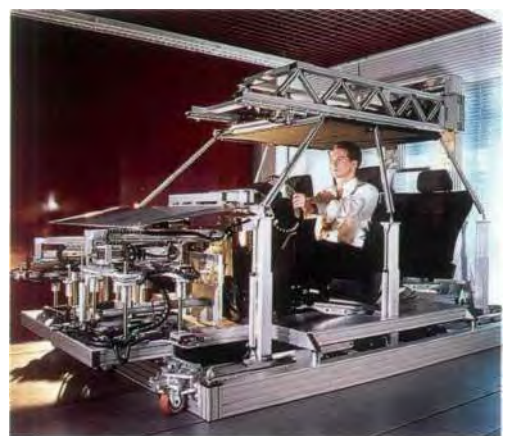
The new ergonomic test rig provides vehicle developers with important information about customer needs.
