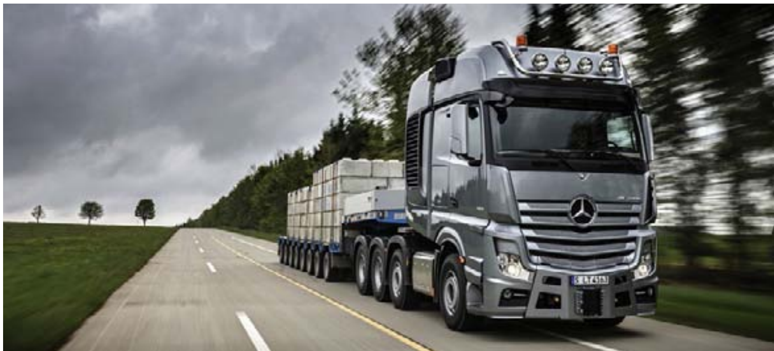
Powerhouse with the star: The Mercedes-Benz SLT – as an Actros or Arocs variant – can pull extra-heavy loads weighing up to 250 metric tons.
