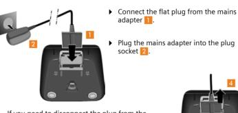
If you need to disconnect the plug from the charging cradle, press the release button 3 and disconnect the plug 4.
