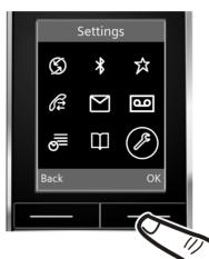
▶ Using the control keys, navigate right, left, up and down 🔁 until the submenu Settings is selected.
