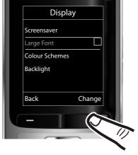
▶ Press down on the control key ☐ until the Large Font menu option appears on the display.
