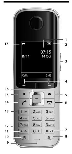
Illustration of handset on a base with SMS functionality.
