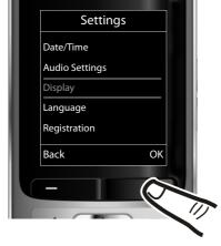
▶ Press down on the control key ↓ until the **Display** menu option appears on the display.
