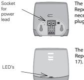
The power lead supplied is plugged into the socket on the Gigaset Repeater's rear side. Using the specified measurements, drill the necessary holes in the wall to mount the device using the screws and plugs supplied.
