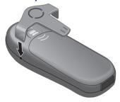
Push the belt clip onto the back of the handset until the side "protrusions" click into place.
