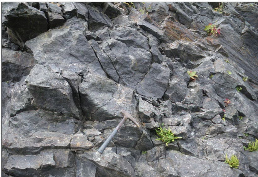
Dolerite, fractured from blasting, conformable with country rock (top right).
