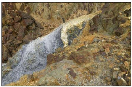
Exposure of massive sulphide mineralization at northeastern end of Cronebane open pit.
