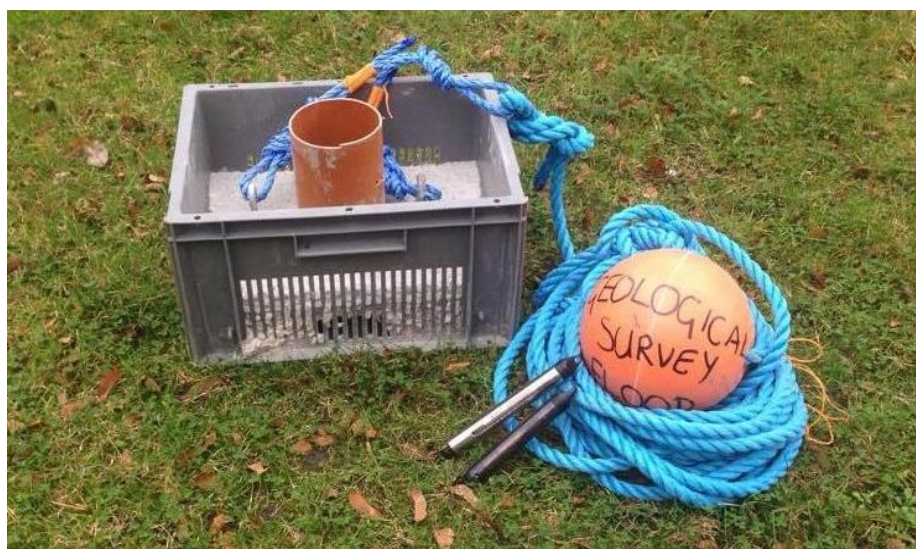
Figure 6: Exploratory monitoring equipment. Custom built monitoring box and Solinst Levelloggers used for data recording.
