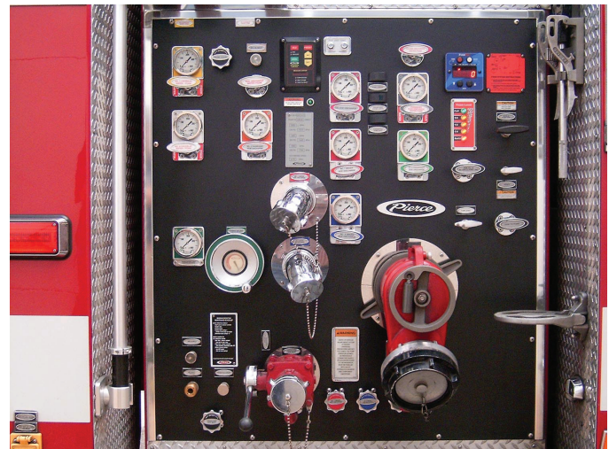
Figure 5 – Color-Coded Control Valves on a Fire Truck (Permission: City of Albuquerque Fire Department)
