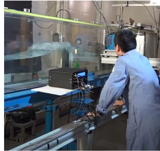
FIGURE 6. A custom wave tank was designed for experiments at the Johns Hopkins University Laboratory for Experimental Fluid Dynamics to study the interactions of waves, oil, and dispersed oil, and the evolution of subsurface oil droplets (C. Li et al., 2017). A piston-type wave plate produces a variety of waves, from rolling ripples to plunging breakers. After an oil slick is introduced, its dispersion is visualized and quantified by high-speed cameras, an illuminating laser, and holography. The tank has been used in various oil spill experiments, including one where aerosolized oil spill chemicals emitted by breaking waves were quantified in support of a health risk assessment for spill response workers (Afshar-Mohajer et al., 2019). Illustration by and used with permission of Cheng Li, Johns Hopkins University. Photo extracted from the Dispatches from the Gulf video and used with permission of Marilyn Weiner, Screenscope Inc.
