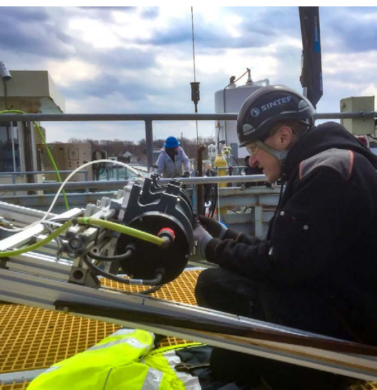
FIGURE 5. The SilCam in situ particle imaging system can distinguish between oil and gas droplets and quantify their distributions from a mixed release, as happened during the DWH incident (Davies et al., 2017). The SilCam (above) has an adjustable path length that ensures all suspended particles in the sample are in focus and utilizes signatures of transmitted light of different wavelengths through each particle to separate oil droplets, gas bubbles, and oil-coated gas bubbles of equal size and shape. The optical configuration is mounted inside of two underwater housings rated to 3,000 m depth. SINTEF senior engineer Frode Leirvik (left) prepares the SilCam for experiments at the Ohmsett National Oil Spill Response & Renewable Energy Test Facility in New Jersey. Both images provided by and used with permission of Emlyn Davies, SINTEF Ocean
