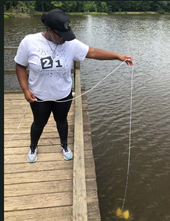
REU student Andria Miller deploys her homemade plankton net (left) and Secchi disk (right), and measures chemical water properties (middle) using test strips. Note: The photos were staged without a life vest, although one was worn during actual sampling.
