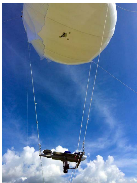
FIGURE 4. The complex processes in the upper ocean—which drifters, ships, and satellites have limited ability to observe—are relevant to oil drift and spread. To better understand near-surface ocean currents, the Ship-Tethered Aerostat Remote Sensing System (STARSS) was custom outfitted with a 50.6 MP camera (300 × 200 m field of view) and launched from a research vessel in the Gulf of Mexico to take images of floating bamboo plates every 15 s for 4 h. The data collected provided the first modern in situ observations of small-scale surface dispersion, and results improved diffusivity estimates at the 3–40 m scale, which can enhance the parameterization of ocean transport models (Carlson et al., 2018). Both photos by and used with permission of Tamay Özgökmen, University of Miami
