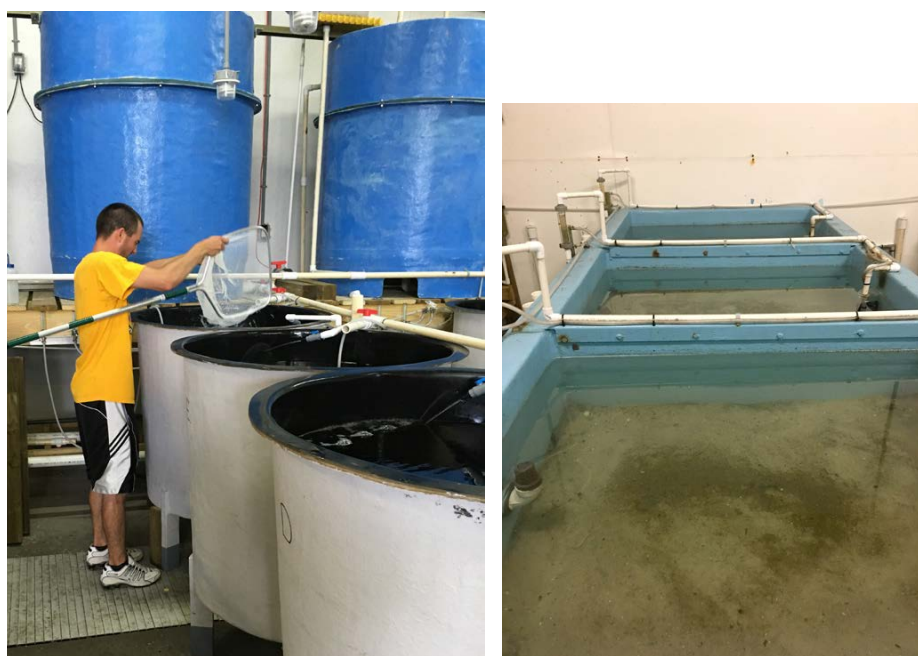
FIGURE 7. Laboratory experiments were designed to investigate oil-induced effects on fish to better understand the impacts of oil spill contaminants on marine life. (left) A new aquatic experimental system with nine 500 L fiberglass tanks (blue tanks contain oil and dispersant mixtures) was used to study short- and long-term sublethal impacts of oil spills on Florida pompano, red drum, and southern flounder. To maintain appropriate water quality and chemistry parameters, the tanks are linked to an aquaculture system that provides recirculating filtered water, and sumps are used to remove oil and dispersant (Main et al., 2018). (right) Nonlethal biomarkers for oil exposure and oxidative stress and damage in southern flounder were investigated using a new experimental flow-through system composed of nine 552 L tanks containing oiled or control sediment (Sherwood et al., 2019). Both photos by and used with permission from Kevan L. Main, Mote Marine Laboratory
