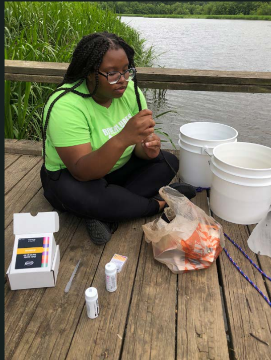
REU student Andria Miller deploys her homemade plankton net (left) and Secchi disk (right), and measures chemical water properties (middle) using test strips. Note: The photos were staged without a life vest, although one was worn during actual sampling.
