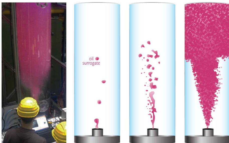
FIGURE 5. Scientists and engineers evaluate droplet size distributions from oil and gas jet experiments using a surrogate (pink stained) oil. For more information, see Pesch et al. (2020). Left photo courtesy of Michael Schlüter, TUHH, Hamburg, Germany
