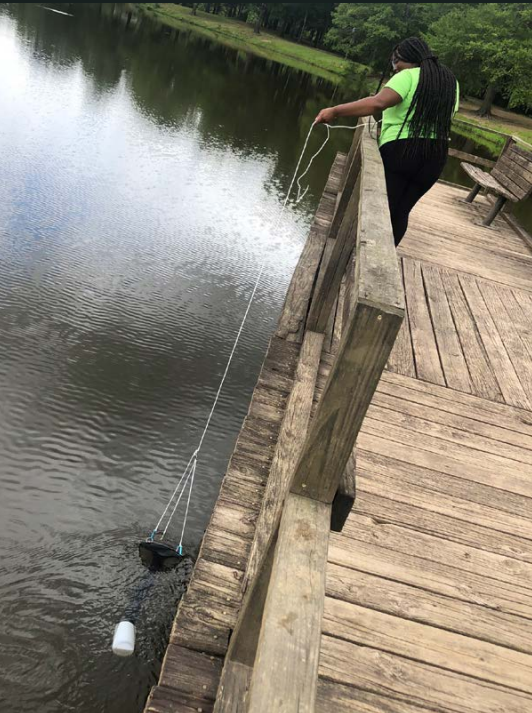
REU student Andria Miller deploys her homemade plankton net (left) and Secchi disk (right), and measures chemical water properties (middle) using test strips. Note: The photos were staged without a life vest, although one was worn during actual sampling.
