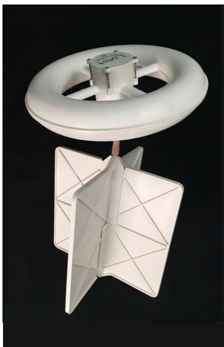
FIGURE 3. During the DWH incident, a need was revealed for more accurate information about the influence that complex upper-ocean currents have on oil transport. To better understand these fast-moving, short-lasting currents, field experiments were conducted in the Gulf of Mexico and used the new Consortium for Advanced Research on Transport of Hydrocarbon in the Environment (CARTHE) drifter, which is easy to assemble, has a low production cost, and is biodegradable (Novelli et al., 2017). The drifter is made from a polymer produced by sugar-fed bacteria. A global positioning system and alkaline batteries are housed in its floating torus, and a four-sail drogue attached to the torus with a flexible connector keeps the floater upright on waves (see photo on opening page of this article). During field experiments, the CARTHE drifters clustered along fronts, and then later dispersed, suggesting that floating oil might accumulate similarly and identifying a possible window of opportunity for a targeted deployment of resources during a spill response (D'Asaro et al., 2018). Image by and used with permission of Cédric Guigand, University of Miami
