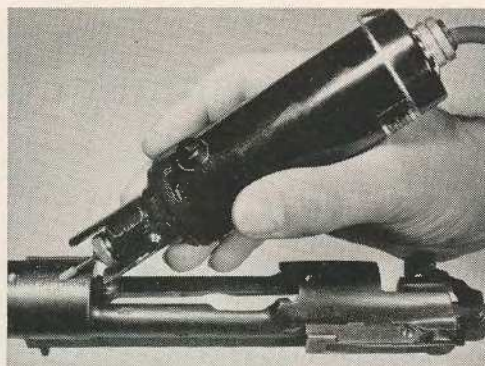
Grinding a starting spot on hard actions assures precise hole location. Right: Grit-treated felt bobs prepare the hard-to-reach spots for bluing.
