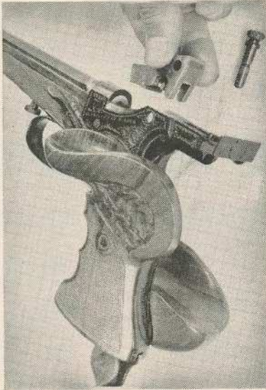
The Record Match pistol uses modified Martini-type action.
