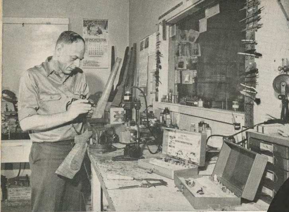
Author uses the compact electric grinder and rotary files on much of his stock inletting.
