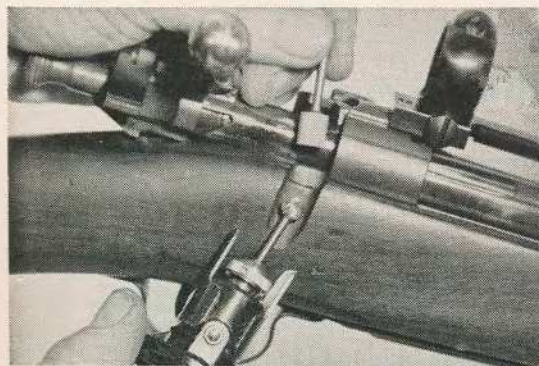
Rotary file cuts bolt notch in the stock; stone is used on the action.
