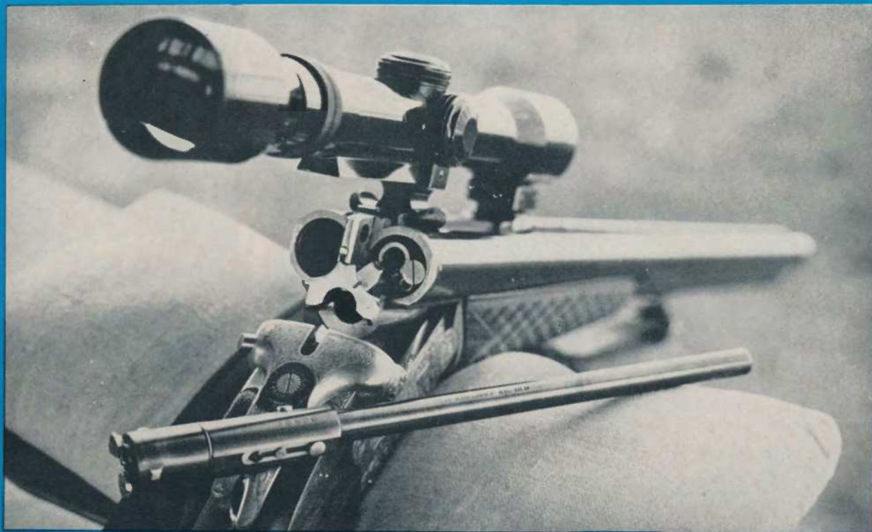
Mounted in a drilling, the Krieghoff .22 barrel inserts increase the gun's effectiveness. Easily adjustable, they can be mounted to use the same sight setting for 40 yard shots as the larger bore does at 200 yards.
