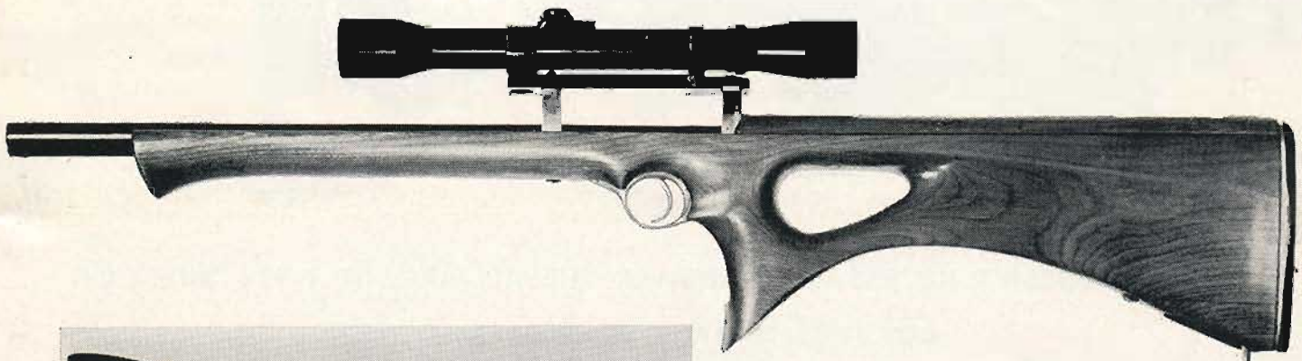
Built on BSA Martini action, this .218 Bee is less than 30 inches long, yet has a 26" barrel. Birch stock is streamlined, makes gun look longer than it measures.
