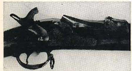
Modified Springfield muzzle loader permits the use of metallic ammo.
