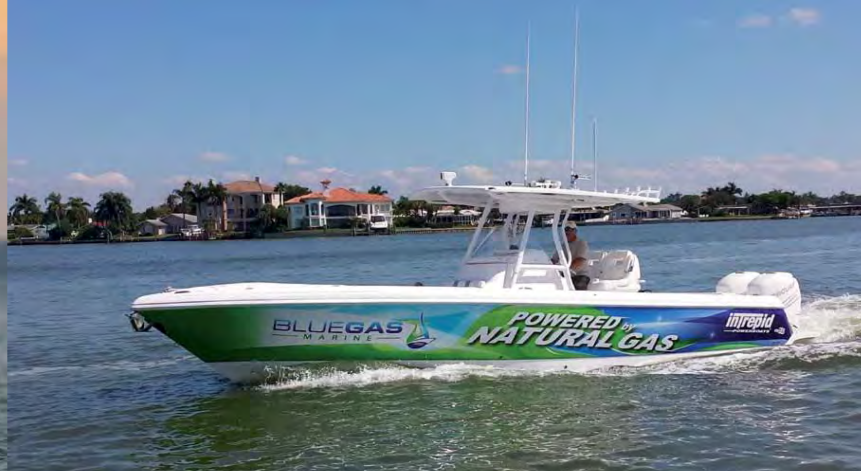
Bluegas Marine worked with boat maker, Intrepid, and engine giant, Mercury to build a Natural Gas powered 30-foot center console. The fuel eliminates fumes and odor, is 25% cleaner than gasoline and cost only $1.50 a gallon. Storing natural gas takes 2-3 times more space than liquid gasoline. Boaters can switch from gasoline to natural gas at the push of a button without even cutting off the engines. Opposite: The radical new Evinrude E-TEC G2 has been completely redesigned on the inside as well as the outside.
