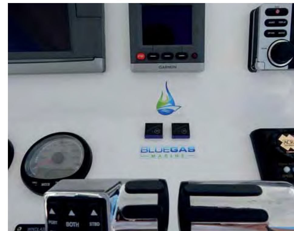
Bluegas Marine worked with boat maker, Intrepid, and engine giant, Mercury to build a Natural Gas powered 30-foot center console. The fuel eliminates fumes and odor, is 25% cleaner than gasoline and cost only $1.50 a gallon. Storing natural gas takes 2-3 times more space than liquid gasoline. Boaters can switch from gasoline to natural gas at the push of a button without even cutting off the engines. Opposite: The radical new Evinrude E-TEC G2 has been completely redesigned on the inside as well as the outside.
