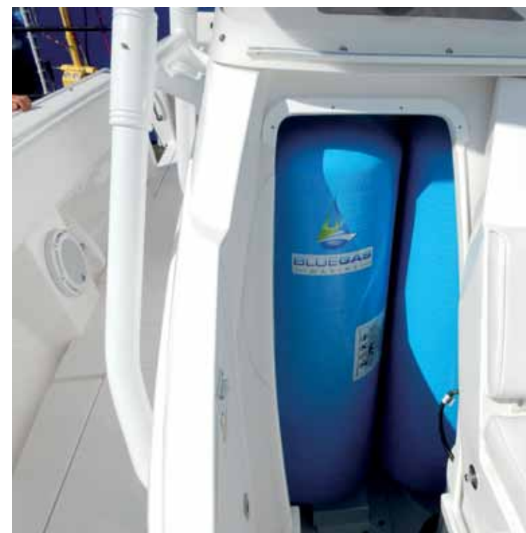
Bluegas Marine worked with boat maker, Intrepid, and engine giant, Mercury to build a Natural Gas powered 30-foot center console. The fuel eliminates fumes and odor, is 25% cleaner than gasoline and cost only $1.50 a gallon. Storing natural gas takes 2-3 times more space than liquid gasoline. Boaters can switch from gasoline to natural gas at the push of a button without even cutting off the engines. Opposite: The radical new Evinrude E-TEC G2 has been completely redesigned on the inside as well as the outside.
