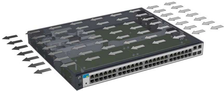
Figure 2-1. Air flow direction of the E2620 switches
