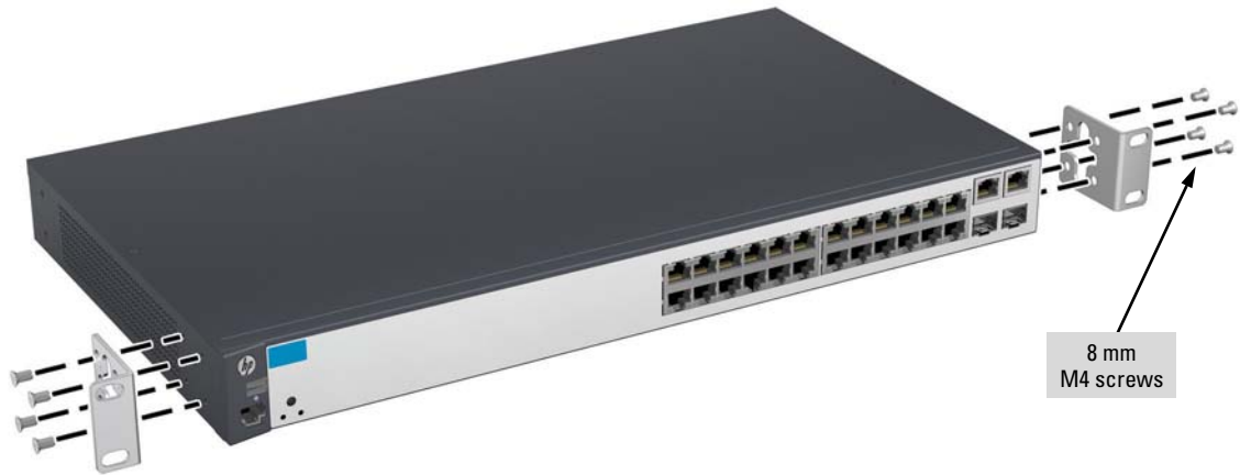
Figure 2-7. Attaching small mounting brackets
