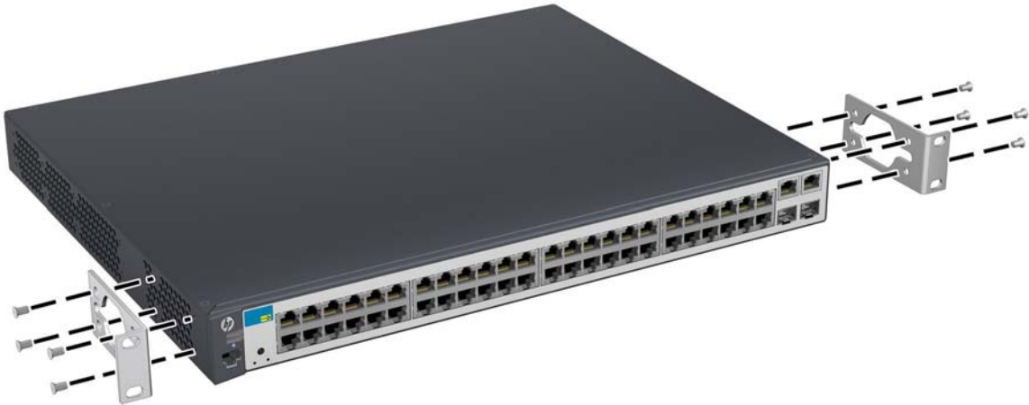
Figure 2-5. Attaching large mounting brackets
