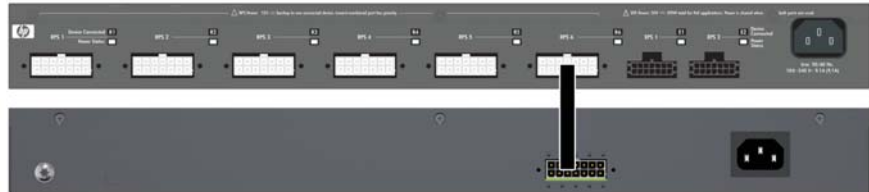
Figure 2-15. Connecting RPS to one switch
