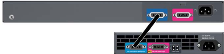
Figure 2-17. Connecting the 630 RPS to a switch
