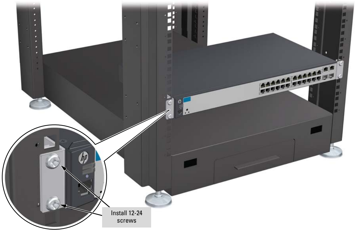
Figure 2-8. Mounting in a rack
