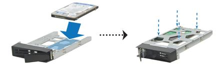
3 Insert the loaded drive tray into the empty drive bay.
