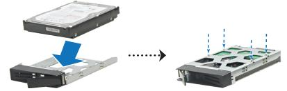
• For 2.5" drives: Place the drive in the drive tray. Turn the tray upside down and tighten screws into the four spots indicated below to secure the drive.
