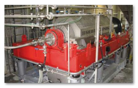
The DZ series can also be supplied in a vapor-tight and gastight design. For these applications, the product housings are manufactured in two pieces and sealed with chamber rings. The geometry of the rotating parts is designed for the specific separation requirement.
