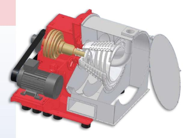
In the traditional design, the complete rotor unit is installed in a large bearing housing. The drum and the worm are overhung into the product collection housing.
