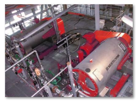
Decanters of the TS series are typically used in gastight process systems.
