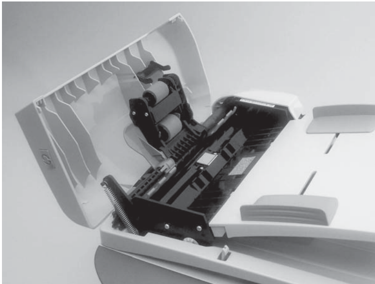
Figure 5-20 Replacing the ADF pickup roller assembly (1 of 6)
