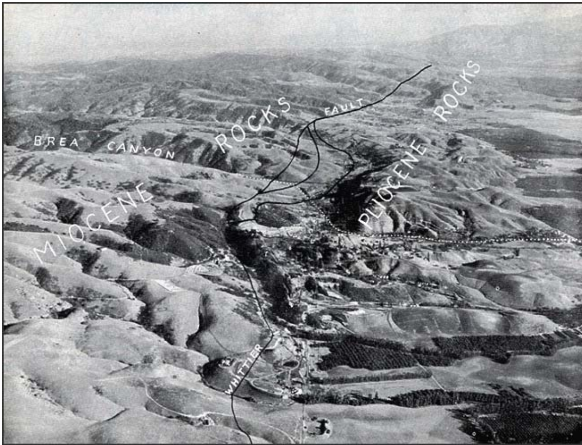
Figure 5a: Photograph of the Whittier Fault (toward southeast). The Miocene and Pliocene rocks labeled in the photo are the thick sedimentary rock layers laid down between ~13 and 2.5 Ma that form the roof rock of the Puente Hills. (Original Photo by J.S. Shelton and R.C. Frampton, in Bennie W. Troxel, "Geologic Guide No. 3, Los Angeles Basin," In Geology of Southern California , Richard H. Jahns, ed., California Division of Mines Bulletin 170 (San Francisco: Department of Natural Resources, 1954), 28.)
