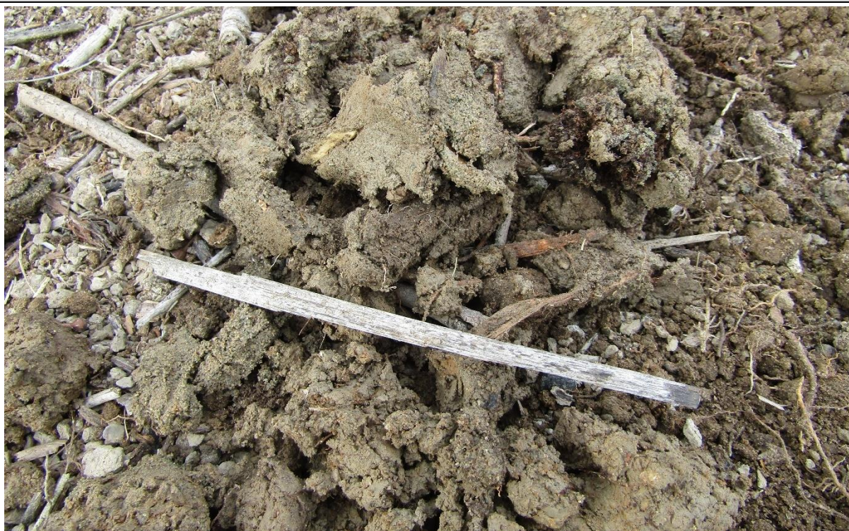
1.13. Example of wetland no. 1 soil sample (gleyed and mottled conditions).
