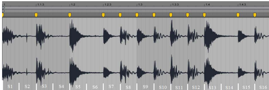
Fig. 1. Time domain visual representation of the first bar of a drum break in Melvin Bliss – Synthetic Substitution in Ableton Live environment. Quantized through audio stretching to every 16 th note. The markers are called Warp Markers and denote transients that were time shifted — in our nomenclature these are the events of the drum break.
