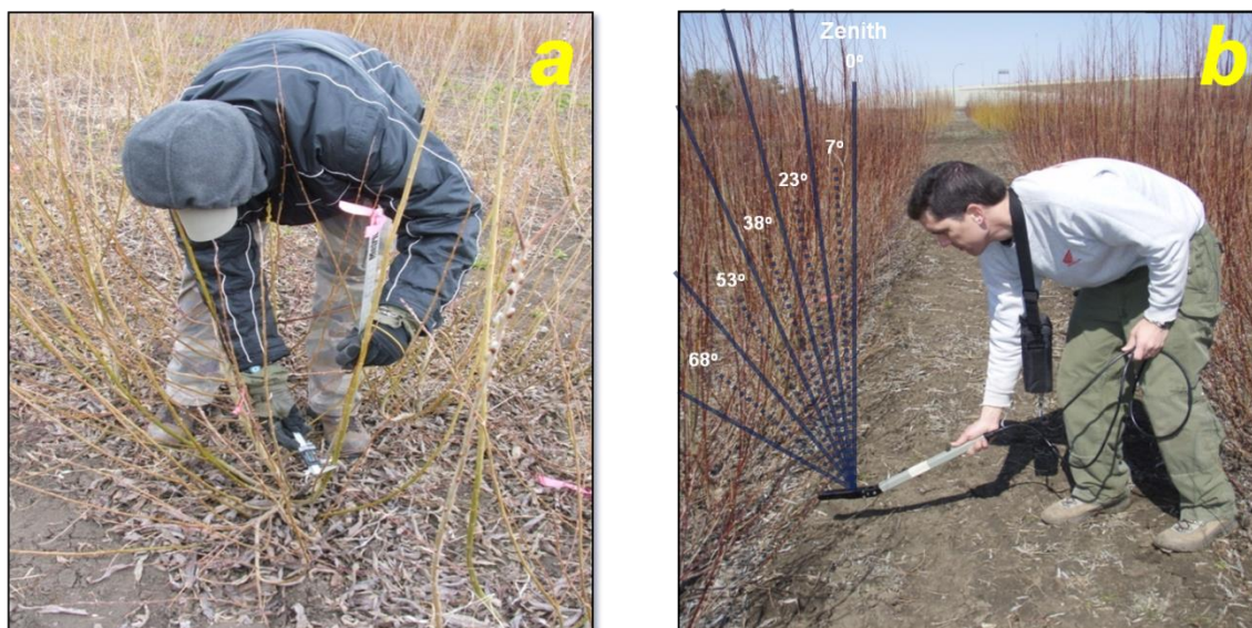
Figure 1. Estimating above-ground willow biomass using an allometric technique (a) and a LAI-2000 Plant Canopy Analyzer to measure the ‘gap fraction’ (i.e., fraction of the sky visible from beneath the canopy) corresponding to five sensor rings centred on different zenithal angles (b).
