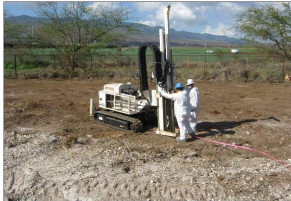
Figure C-18. Use of direct push rig to collect increment cores from subsurface DUs.
