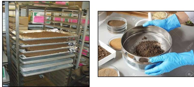
Figure-K-1. Air drying and sieving of samples.
