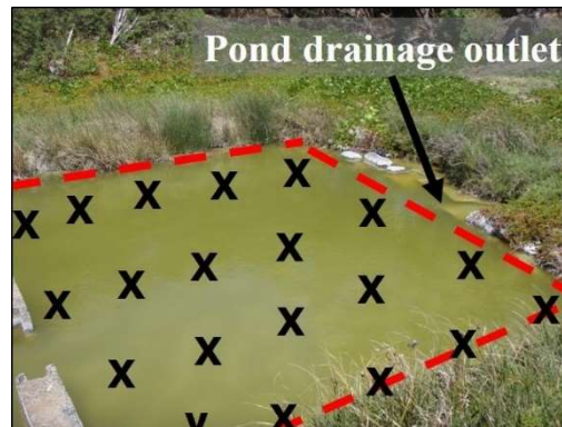
Figure C-30. DU designated for characterization of sediment at the mouth of a wastewater pond outfall. "X" indicates sample increment collection locations.
