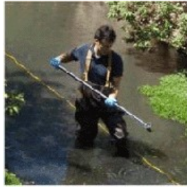
Figure J-3. Alternative scoop-shaped samplers for thin sediment layers.
