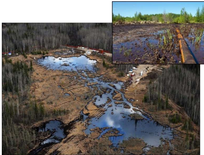
Figure C-25. Release of light crude oil into a marsh from a broken pipeline.
