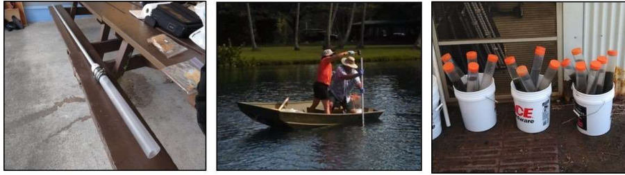
Figure J-4. Use of prefabricated, manual core sampling device to collect sediment increments.
