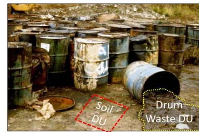
Figure C-15. Designation of small, targeted DUs within an illegal dump site to identify potential contaminants of concern.
