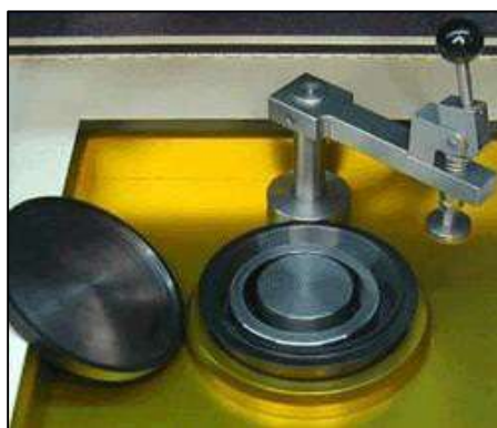
Figure K-4. Puck and ring mill, used to crush small masses of soil to very fine, consistent grain size.
