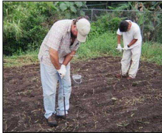
Figure F-3. Multi Increment Sample Collection Collect an "increment" of soil at each point. In this example (very soft soils), a sampling tube is used to extract a cylindrical volume of soil to a depth of approximately 10 cm. Each increment typically weighs 20 to 50 g. Subsequent increments for the target DU are placed in the same container.
