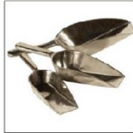
Figure J-3. Alternative scoop-shaped samplers for thin sediment layers.
