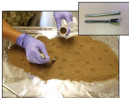
Figure-K-3. Manual collection of subsamples in the laboratory.
