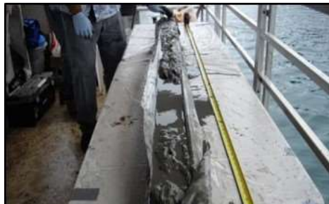
Figure J-10. Removal of increment core from Vibracore sampling tube and preparation for subsampling. Bulk Multi Increment sample prepared by combination of increment subsamples from all cores collected within the targeted DU.
