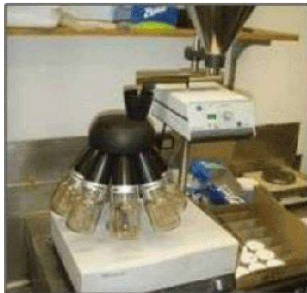
Figure K-2. Use of a sectorial splitter to collect laboratory subsamples from bulk Multi Increment field samples.
