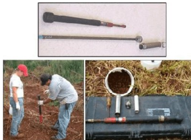
Figure F-13. Use of a Slide Hammer to Collect Soil Increments.
