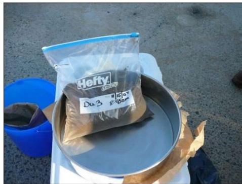
Figure F-5. Increments combined to prepare a 1 to 3 kg Multi Increment sample.
