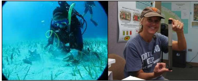
Figure J-11. Diver assisted sediment sample collection.
