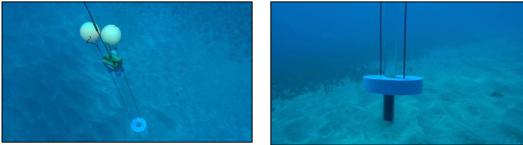
Figure J-6. Submersible platform used to collect sediment increment cores within a targeted DU (manufactured by Specialty Devices Inc.).
