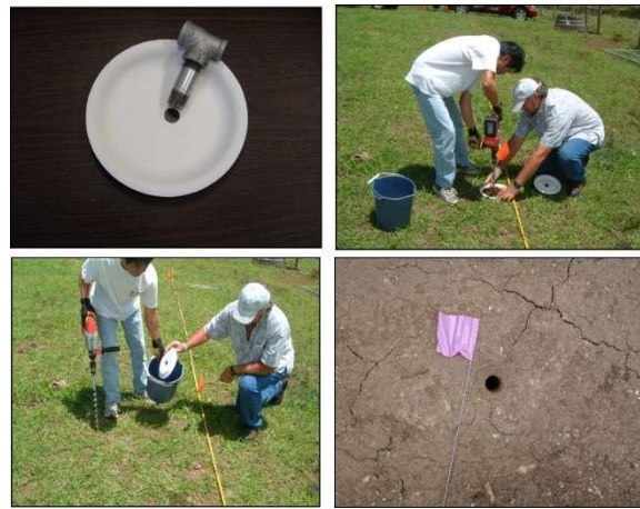
Figure F-10. Use of cordless drill for sample collection.
