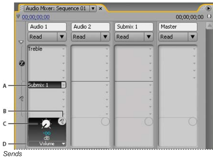
A. Name of submix assigned to send, and Send Assignment menu B. Send mute C. Control knob for selected send property D. Send Properties menu
