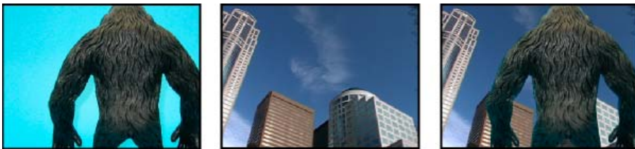
Nonstandard blue screen (left) and background (center) are combined with Color Key effect (right).
