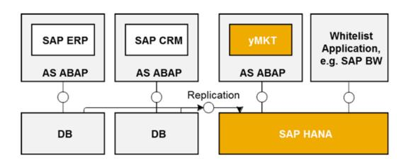
Figure 6: Hub-Deployment with Shared SAP HANA System of Other Application
