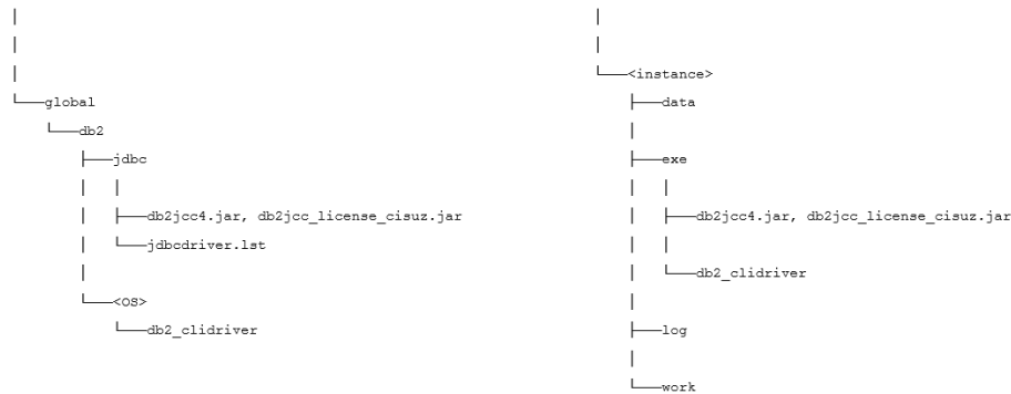
Directory Structure of the Database Client for SAP NetWeaver (including the JDBC Driver)
