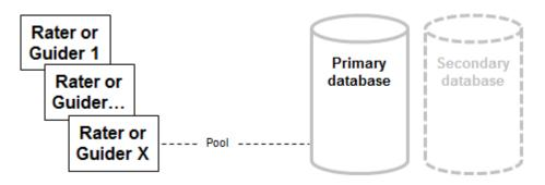
All the running services are associated to the primary database. In case of failure of this primary database, all resources are taken back by the secondary database, which makes them available again. Every server instance of the SAP CC system which was connected to the primary database automatically reconnects to the secondary database, in order to ensure the availability of the charging operations.
