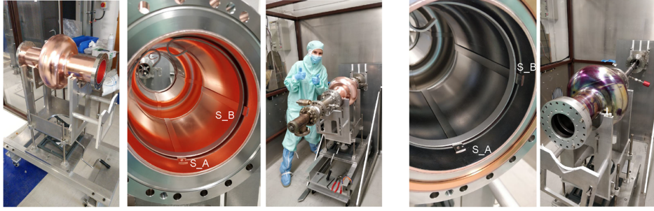
Figure 4.15.: First Nb thin-film-coated 802 MHz cavity at CERN. The three leftmost figures show the copper cavity before coating including the clean-room assembly. The two rightmost figures show the cavity after the Nb coating [226].
