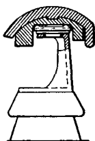
FIG. 44.—Inverted channel third rail.
