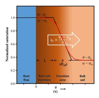
**Figure A1.** Schematics of the root flow–soil boundary and soil moisture transition for the parameterization of horizontal water flux  $q_x$ . The red dashed line represents the analytical solution, and the black-solid line represents the parameterization. Soil moisture is saturated (i.e.,  $\theta_s$ ) in the root–soil boundary (width  $\lambda$ ), and decreases linearly in the transition zone (width  $\delta$ ) before reaching that of the bulk soil ( $\theta_w$ ).
