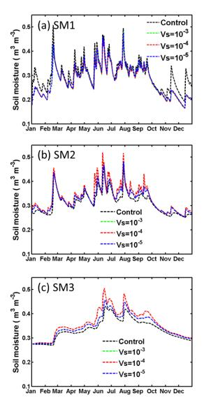
Figure 9. Sensitivity test on  $V_s$  for the LHC case with optimal SLR = 90 % at depths of (a) SM1 (0–20 cm), (b) SM2 (20–70 cm) and (c) SM3 (70–170 cm). The green dashed, red dashed and blue dashed curves are for  $V_s = 10^{-3}$ ,  $10^{-4}$  and  $10^{-5}$  m s<sup>-1</sup>, respectively. Also shown by black dashed curves are the control run results (i.e., SLR = 0).
