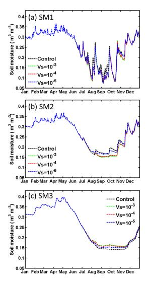
**Figure 10.** Same as Fig. 9, but SLR = 50 % for the HAPEX case at depths of (a) SM1 (0–20 cm), (b) SM2 (20–50 cm) and (c) SM3 (50–160 cm).
