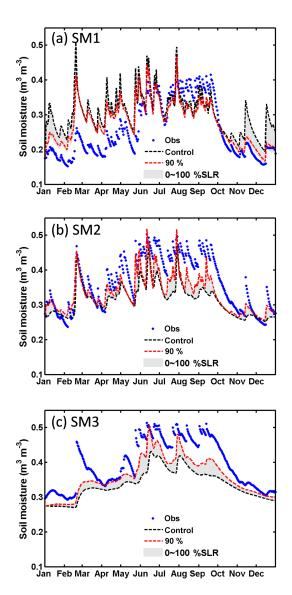
**Figure 5.** Simulated and observed soil moisture for the LHC site at depths of (a) SM1 (0–20 cm), (b) SM2 (20–70 cm) and (c) SM3 (70–170 cm). Observed results are shown as blue dots. Simulations with SLR = 0 (i.e., control run, without stem–root flow) and SLR = 90 % are shown as black dashed and red dashed curves, respectively. The area of grey shading enclosed by SLR = 0 % and 100 % indicates the possible range of the stem–root flow effects. All simulation results are daily averages.
