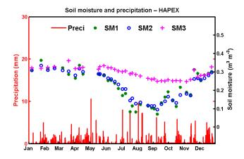
**Figure 3.** The weekly soil moisture (symbols, right axis) and hourly precipitation (red bars, left axis) observed at HAPEX during 1986. SM1, SM2 and SM3 represent the mean soil moisture in the 0–20 cm (green dot), 20–50 cm (blue circle) and 50–160 cm (magenta cross) layers, respectively.
