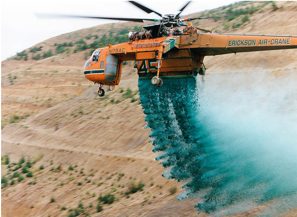
Figure 8.6: A hydroseed mixture can be applied using existing fire-suppression aircraft.
