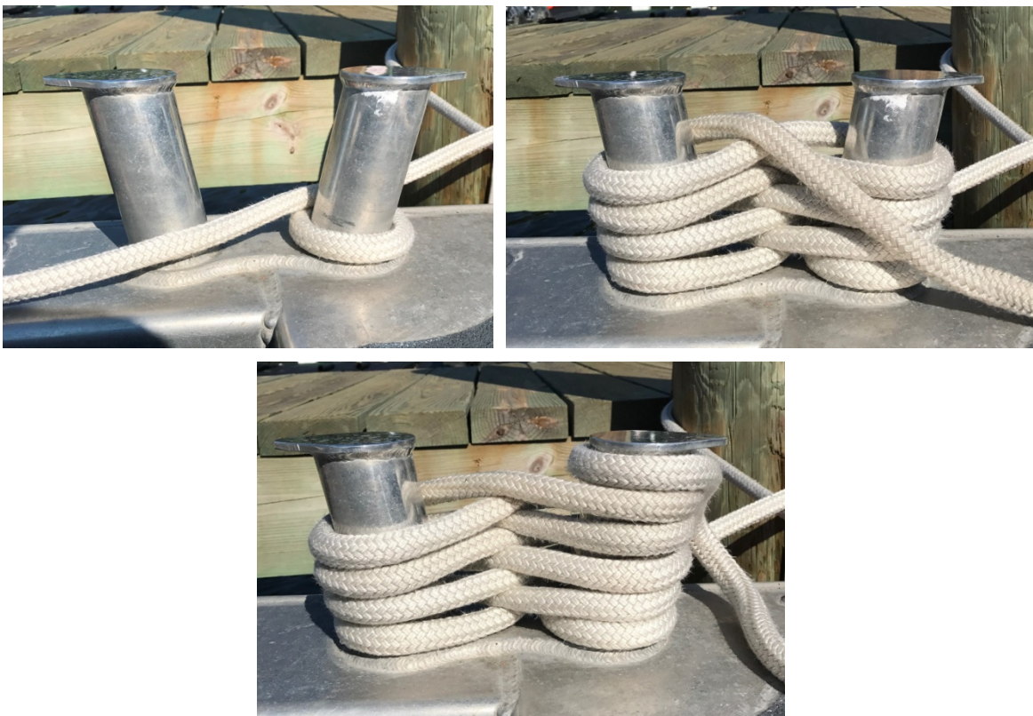
Figure 2-34 Securing a Line to Paired Bitt
