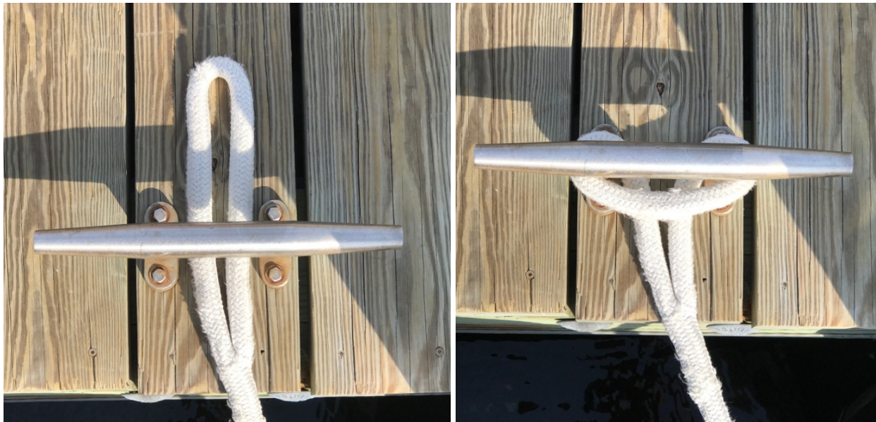
Figure 2-37 Securing a Dock Line to a Cleat
