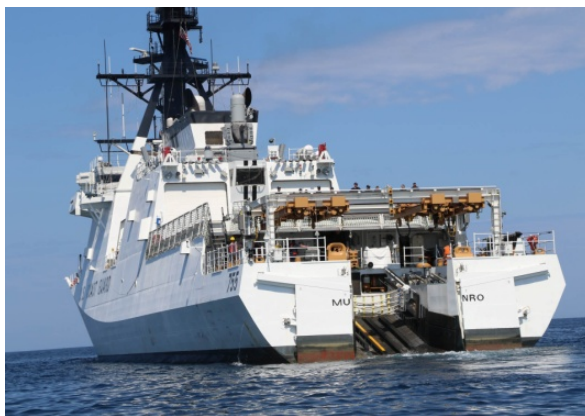
Figure 3-2 Tumble Home Hull Design
