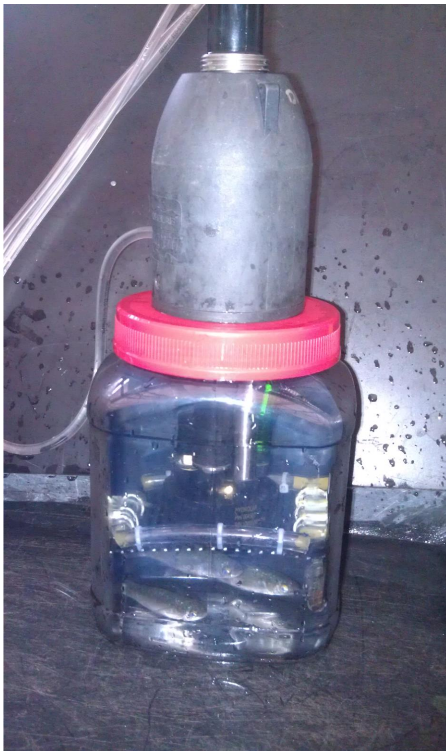
Figure 3- Dissolved oxygen testing quarters with 5 fish and floating mesh, designed for this experiment
