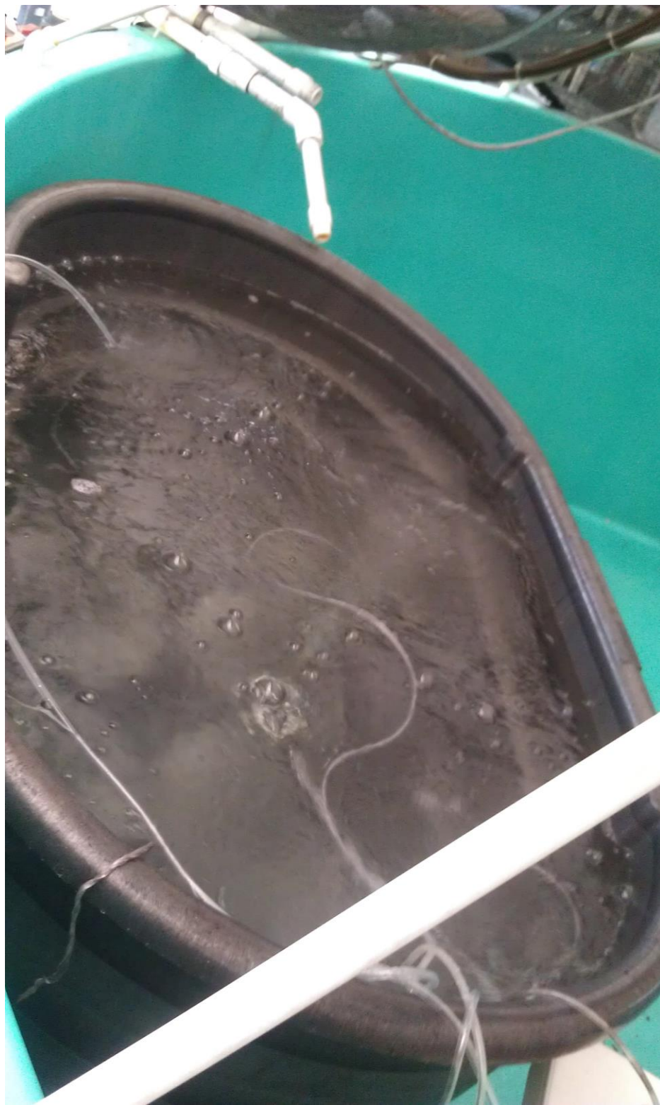
Figure 4- 378 liter water reservoir set up that saturated water to 100% and was used for recovery
