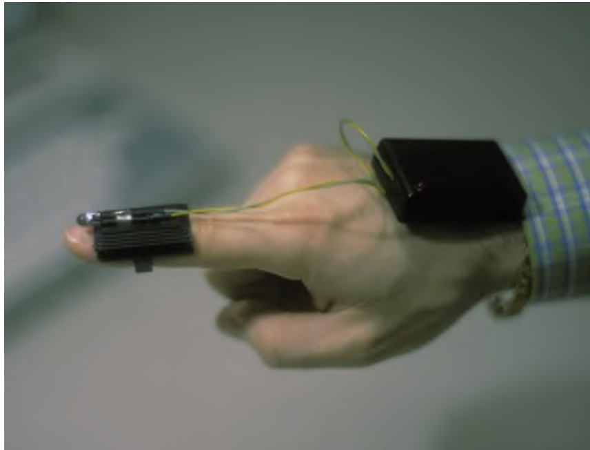
Wearing the finger-mounted emitter. (The black box on the wrist contains batteries and the modulator circuit.)
