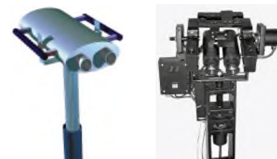
Figure1 The Visorama observation device. An artistic rendering (a). A photograph of the first prototype (b).
